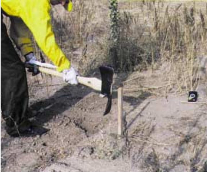
Figure 32—Tool lift height indicator with a stake and colored dowels.
