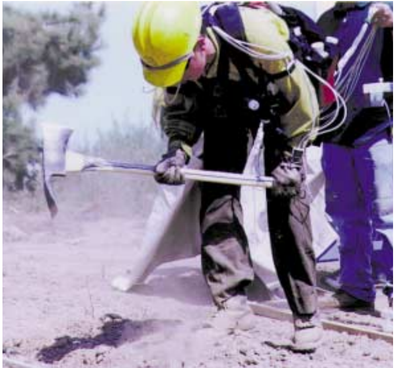
Figure 8—Position/angle sensor mounted on the tool head.
