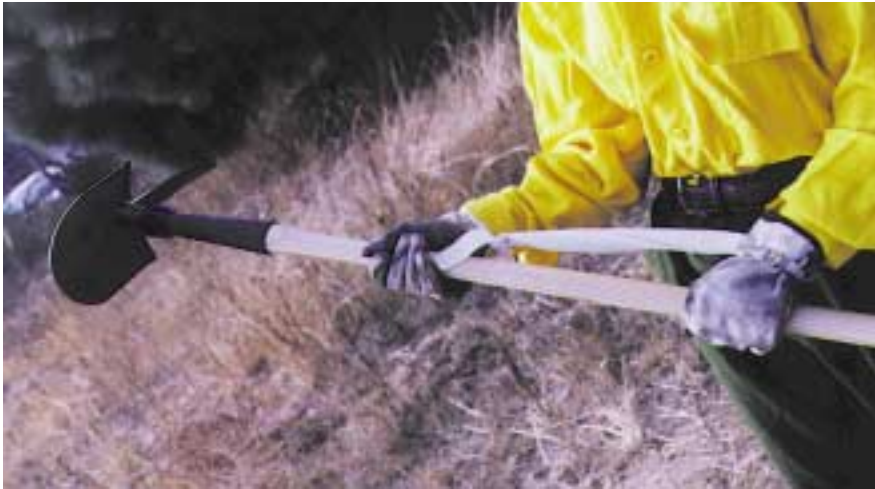
Figure 34—Hand separation maintained within set parameters by elastic cord.
