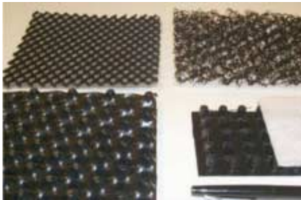
Figure 1—Typical geocomposite drains. The core can vary from a geonet (upper left), a plastic sheet that has been shaped to form cusps (lower left), cylinders (lower right), or mesh (upper right). The pen is provided for scale.
