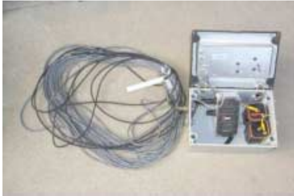
Figure 3—Groundwater level measuring equipment. The piezometer (white cylinder at the end of the cable) measures the water pressure, the datapod (small black box) records the data, and the large outer box powers the piezometer and conditions the electrical signal.
