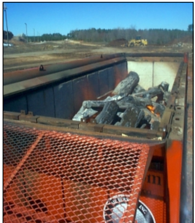
Figure 1—ACD in full operation (no visible smoke).
