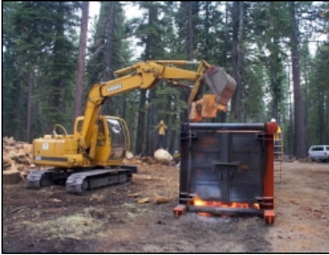
Figure 4—Loading fuel into ACD (full operation).
