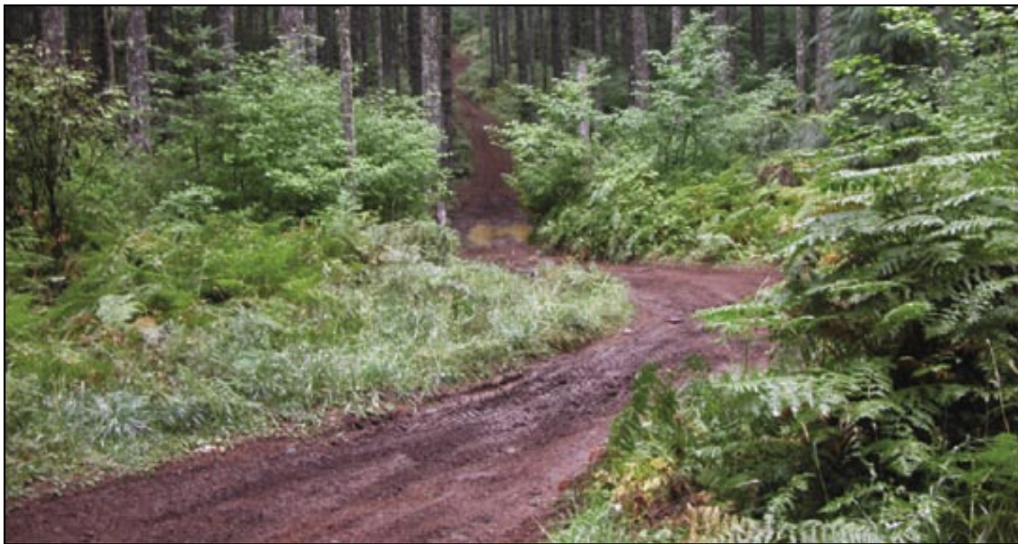
Figure 23—Maintenance level 2 road with single lane and native surface.
