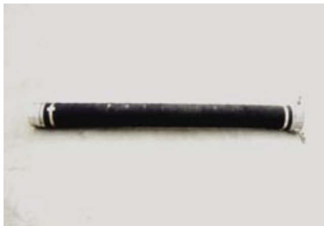
Figure 49—Hose with quick disconnect fittings.
