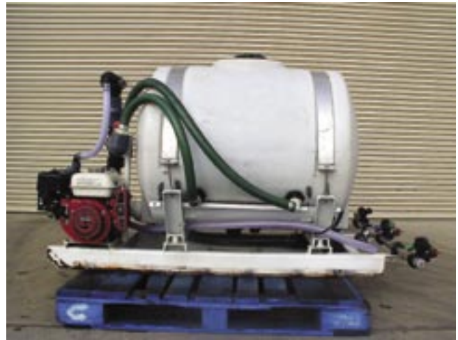
Figure 9—Sprayer module side view.
