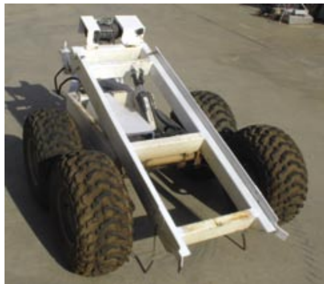
Figure 3–Upper frame, raised, with hydraulic power pack and ram, and battery housing, note winch frame at the top of the photograph.
