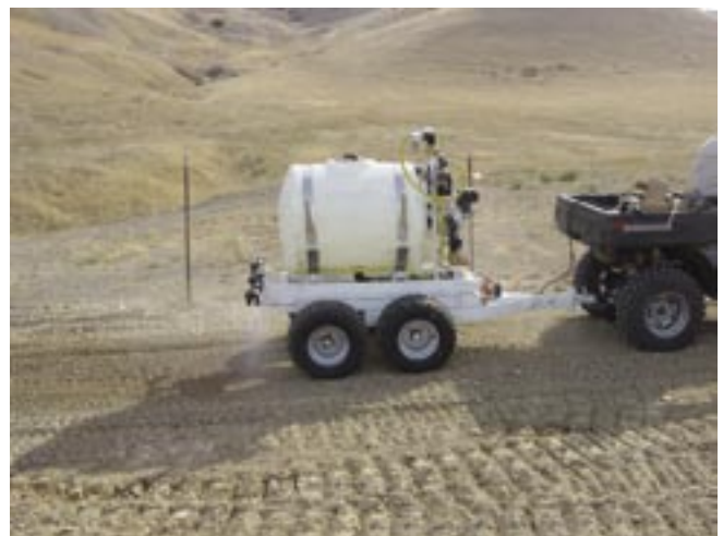
Figure 8—Sprayer used for dust control.
