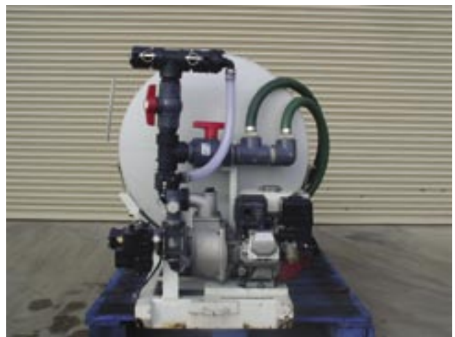
Figure 11—Front view—engine with 2-inch centrifugal trash pump with valves for spray and hydromulch functions.
