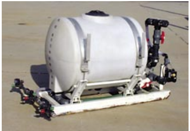
Figure 10—Sprayer module rear view. Note sprayer bar.
