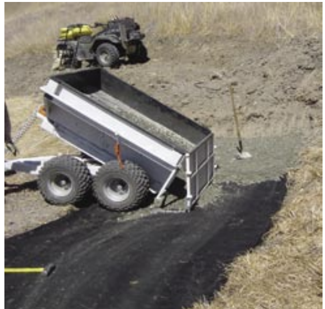
Figure 16— Upper frame raised with dump bed module attached.
