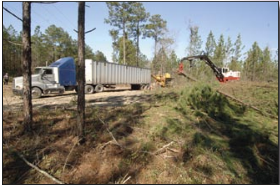
Figure 7-18—Chip-van access into a unit was accomplished by removing the saw logs and then chipping the smaller logs. Once this process is completed, the landing access can be closed and the area subsoiled to improve infiltration.
