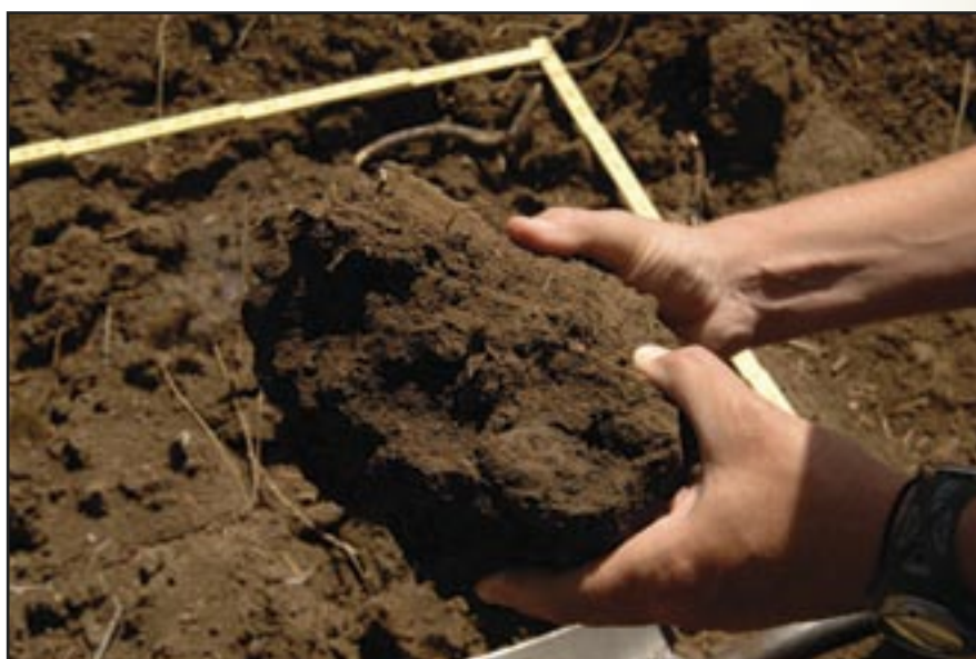
Figure 5-13—An example of the type and size of soil clod created from the equipment.
