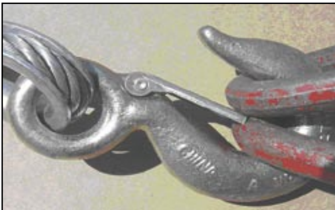
Figure 1—Leadline hook and cargo net links incompatibility.
