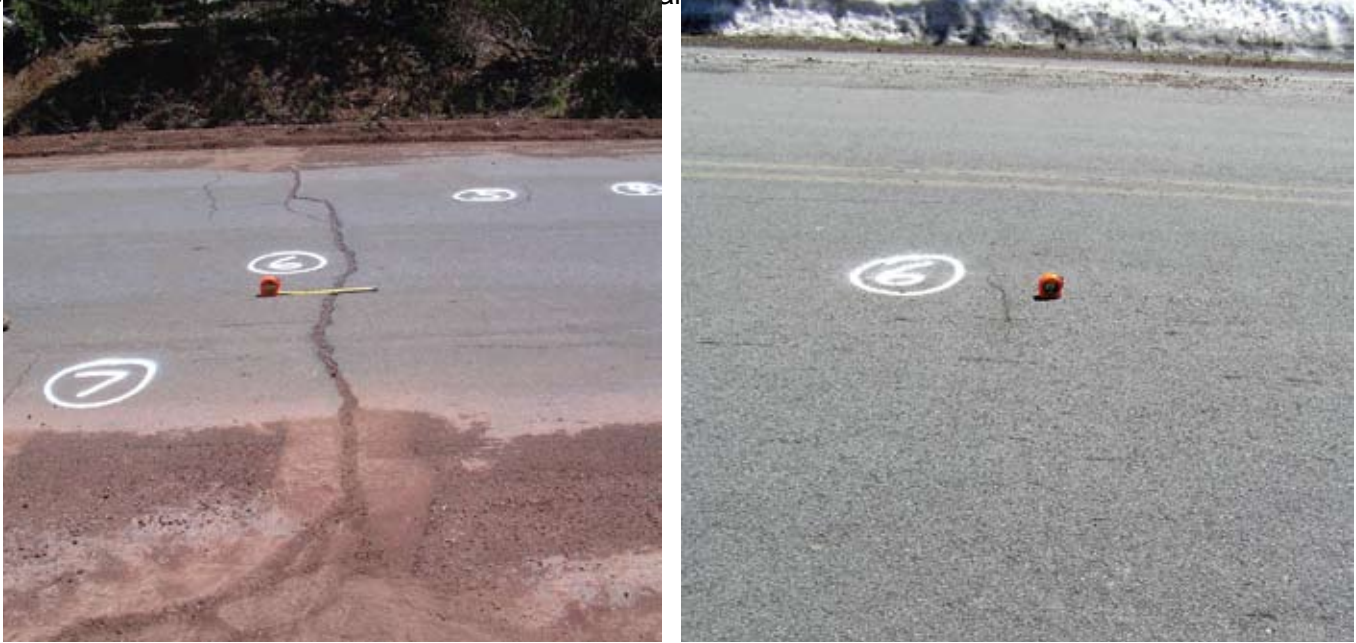
Figure 13—Comparison of reflected crack in GlasGrid-treated cell of test section 1 after 6 years.
