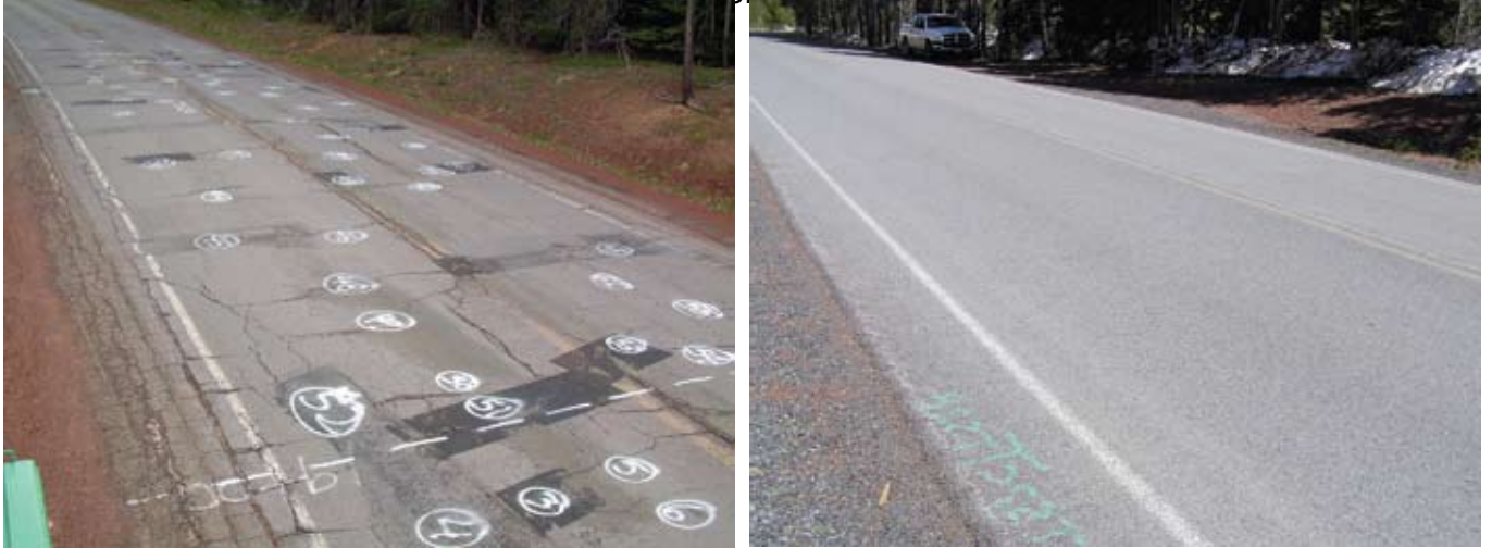
Figure 15—Comparison of test-section 2 surface after 6 years.
