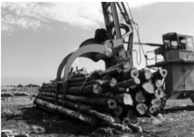
Figure 21. Arms and forks cannot encompass the load after storage. The straps must keep load intact.
