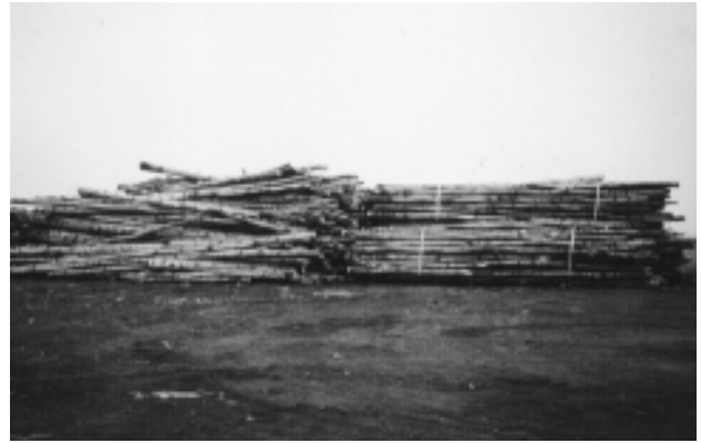
Figure 12. Long view of deck comparing neatness of strapped loads with conventional decking.
