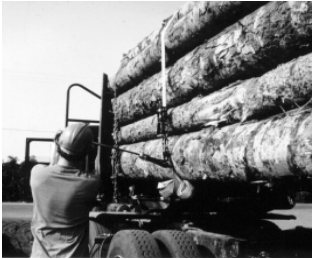
Figure 10. Custom torque wrench used to measure tension.
