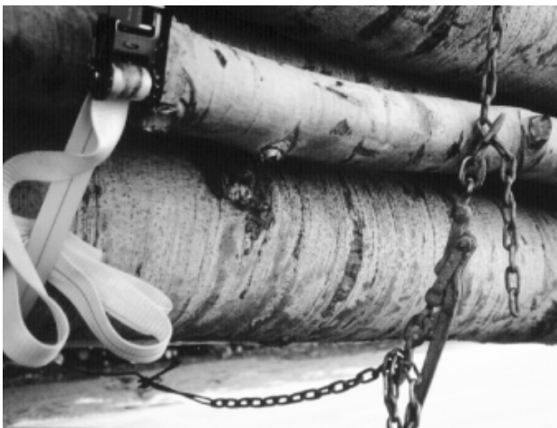
Figure 11. Close-up of strap and wrapper after transport—note how slack the steel wrappers are at the end of the trip.
