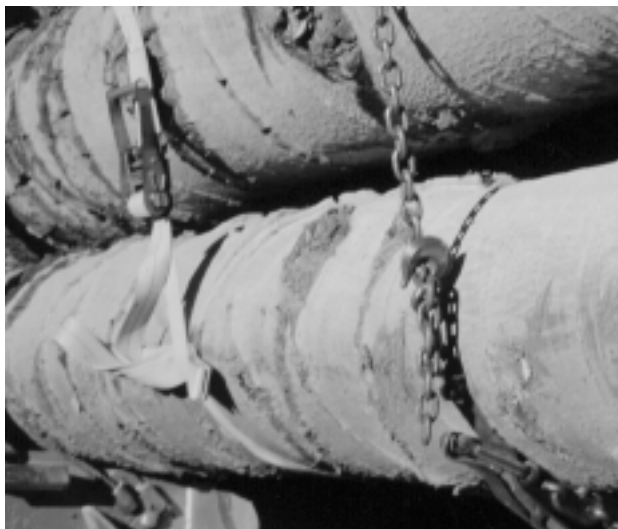
Figure 9. Close-up of strap and wrapper as tensioned prior to transport.
