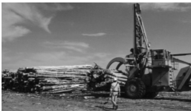
Figure 15. Preparing to release tension by striking winch handle with the shovel blade.
