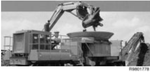
Figure A80. Large tubgrinder, 14 foot diameter tub for large volume grinding. Options include tub magnets, remote control, air compressor, grapple loader, electric models. The Super 14 by EarthSaver Equipment Company Midland, Texas (915) 694-9988.
