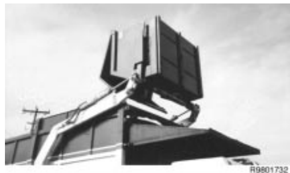
Figure A34. Front load container in open position. The tilted position of the container allows the locking mechanism to unlock; by Capital.
