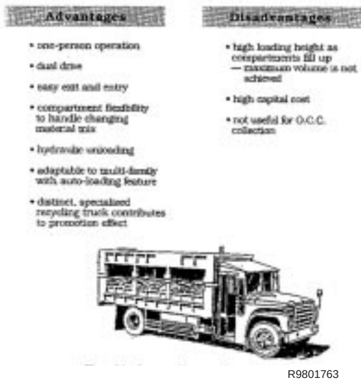
Figure A65. Closed-body recycling trucks, advantages and disadvantages.
