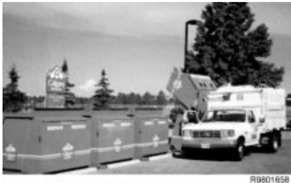
Figure 65. Hyd-A-Ways 4 cubic yard container and hauling truck combination by Haul-All waste container manufacturing company, Canada.
