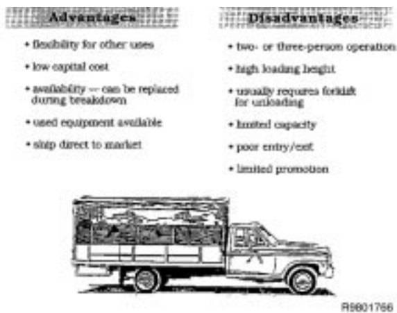
Figure A66. Low-profile closed-body truck, advantages and disadvantages.
