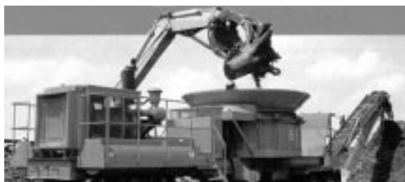
Figure 88. Tub grinder processing green waste materials.
