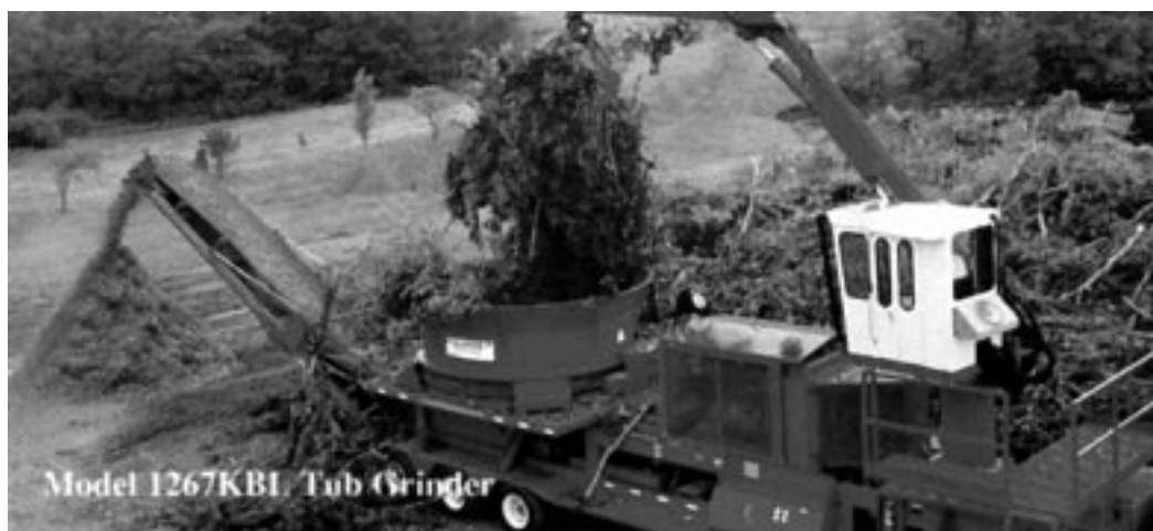
Figure 32. A tub grinder can convert green waste into a compostable mulch mix.
