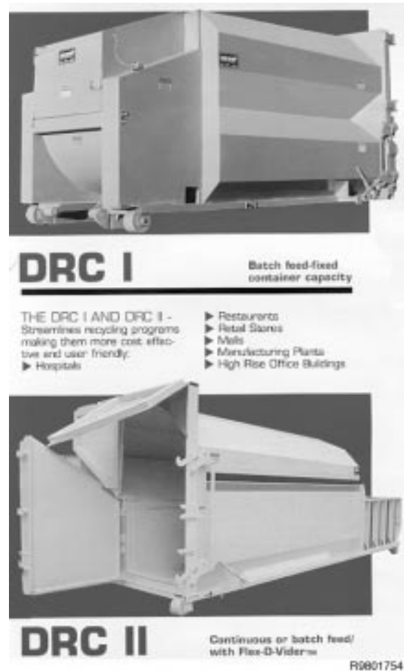
Figure A56. Ramjet dual recycling compactors for wet or dry recycling waste, available in 16 and 22 foot lengths with 20 and 30 cubic yard capacities. Double compartment design completely separate for two types of material (cardboard and aluminum etc.). By Marathon Equipment Company Vernon AL (205) 695-9105 Yerington NV (702) 463-4030
