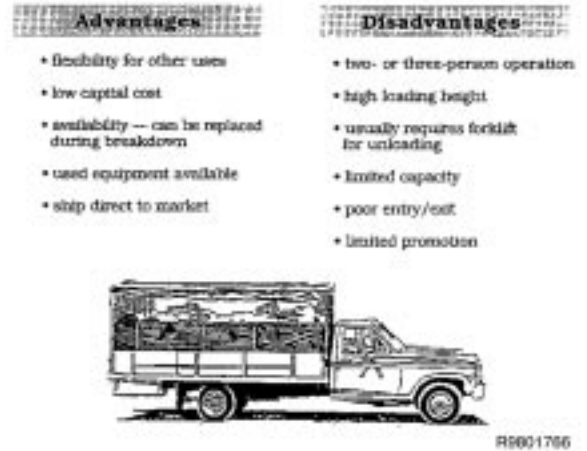
Figure A68. Flat-bed trucks, advantages and disadvantages.
