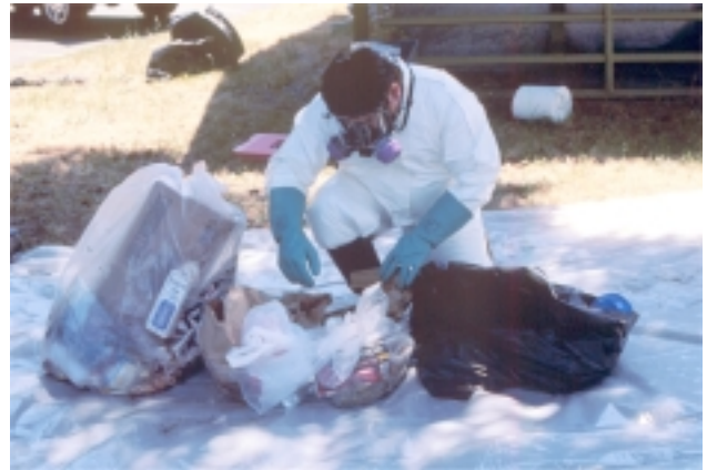
Figure 4. Review of the contents of a 4 cubic yard dumpster at the Six Rivers NF to determine the exact mix of refuse generated by the public. Sources of refuse included local day use sites and campgrounds.
