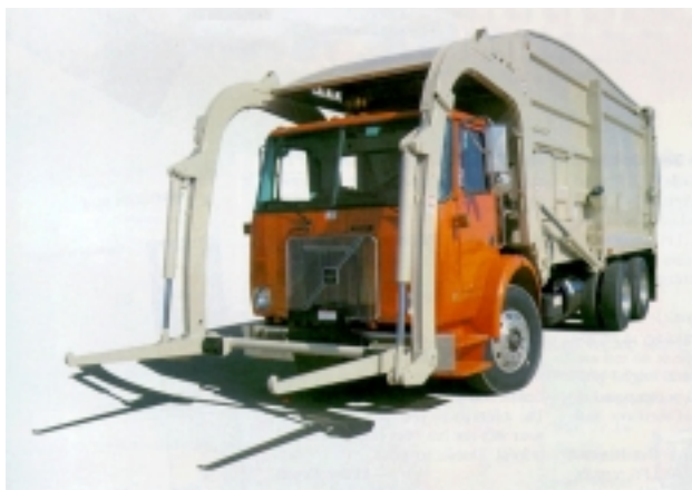
Figure 25. Front loader system, some units can be adapted for dumpsters and 50 gallon plus containers by using a mechanical arm. Photo courtesy of McNeilus Truck and Manufacturing Co.
