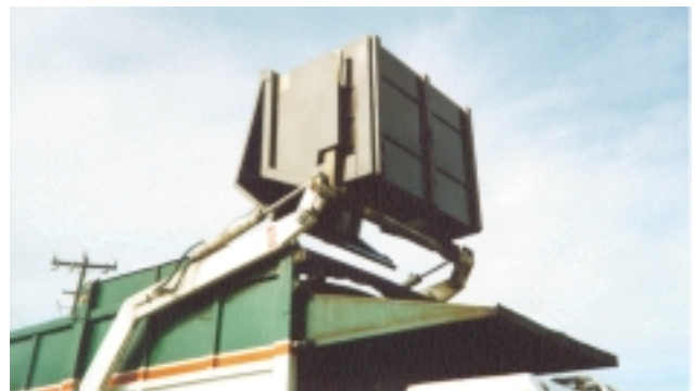
Figure 17. Same as figure 21 but in an unloading position with a typical front-end loader garbage truck. Clearances for this type of operation must be planned for in recreation sites. Photo courtesy of Capital Industries, Seattle WA.
