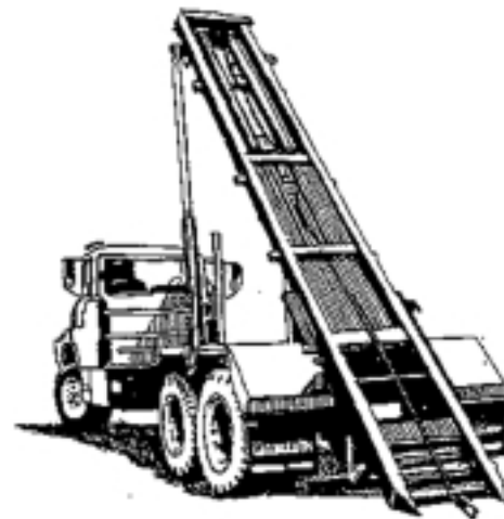
Figure 13. Roll-off trucks require wide turning radius and high tree clearance to drop off and pick up large containers.
