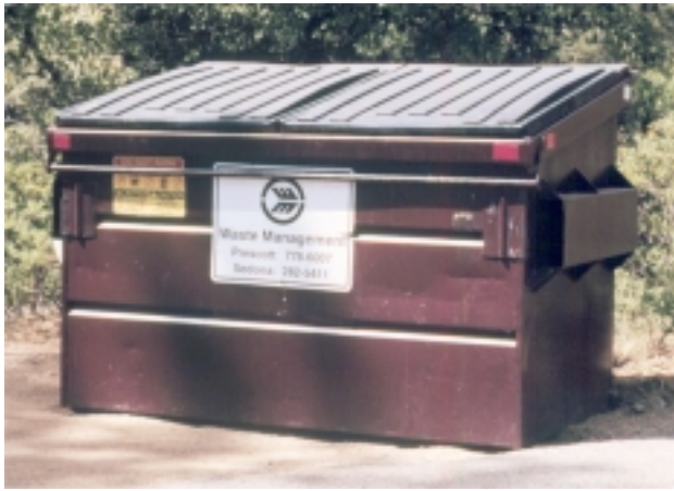
Figure 19. Typical front-load dumpster that can range in capacity from 2 to 4 cubic yards. This particular dumpster is provided by Waste Management Industries.
