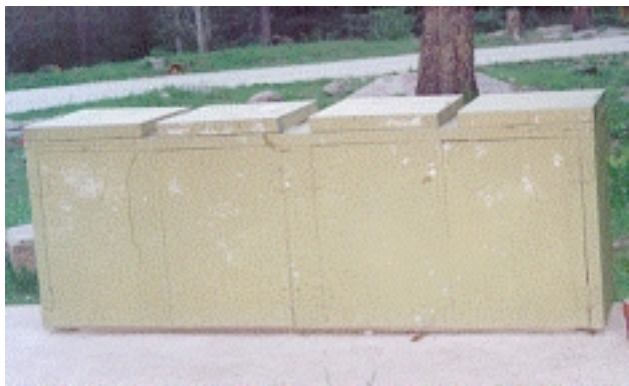
Figure 22. This steel refuse container is often called a four-in-one system. Four 32-gallon individual trash bags are placed inside the container. The refuse is deposited in each of the four hinged access doors and is emptied from the front.
