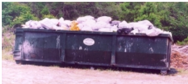
Figure 11. Large capacity roll-off container; these units typically haul 25 to 40 cubic yards of refuse. The unit is picked up by a large flatbed truck and pulled onto the truck with a winch.
