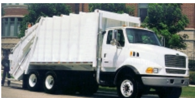
Figure 26. Rear loader also commonly called packer may be loaded without overhead lifting. Photo courtesy of Sterling Truck Corporation.
