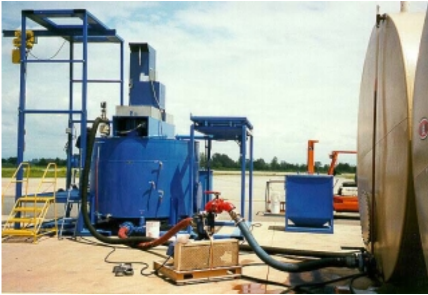
Figure 6—Mixer setup for storage tank reconditioning at Redding Airtanker Base.
