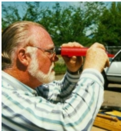
Figure 22—Measurement of retardant salt content using the refractometer.
