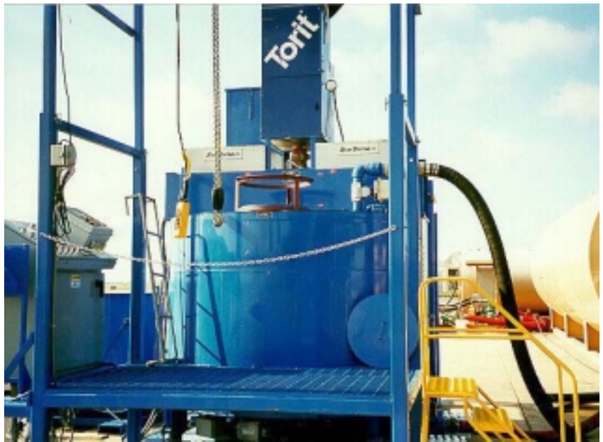
Figure 5—Mixer loading platform with nonskid surface, safety chains and portable stairs with handrails.
