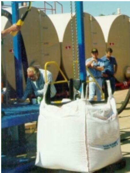
Step 2—Commence bag lifting with the hoist.
