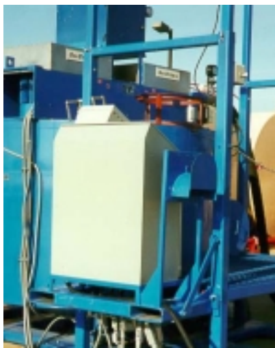
Figure 26—Control console mounting bracket assembly. Notice wiring plug connections at the bottom of the console.
