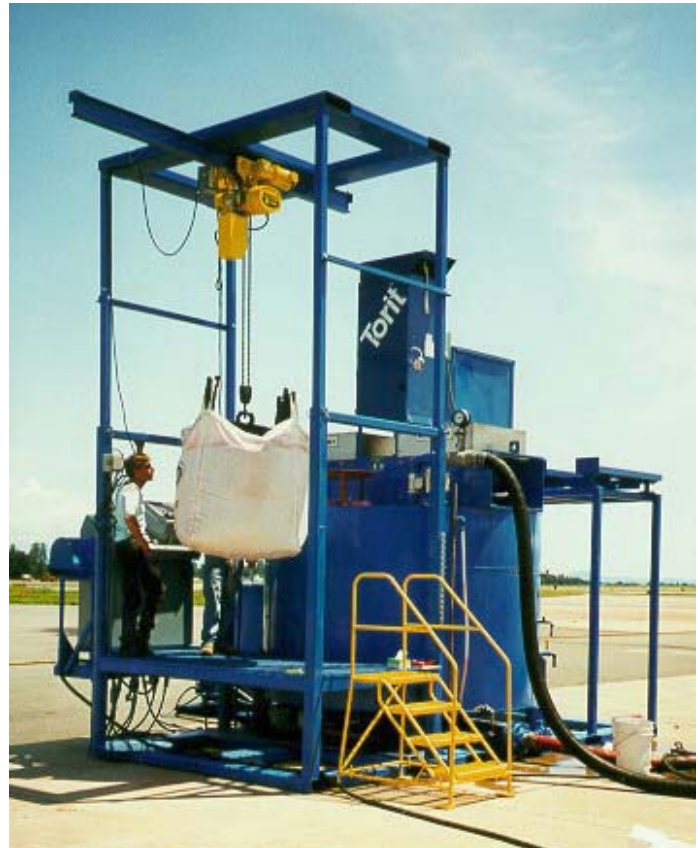
Step 3—Moving bag to mixer with the hoist trolley.
