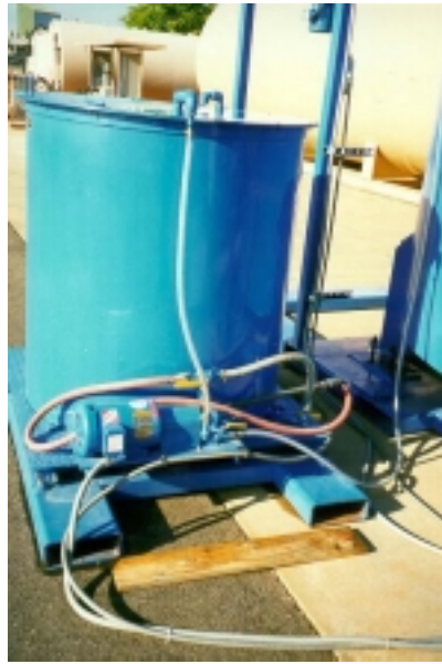
Figure 3—Liquid storage tank and metering pump assembly.
