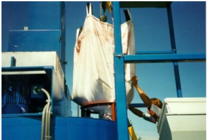
Step 5—Bag positioned on safety ring and bag dumping started.
