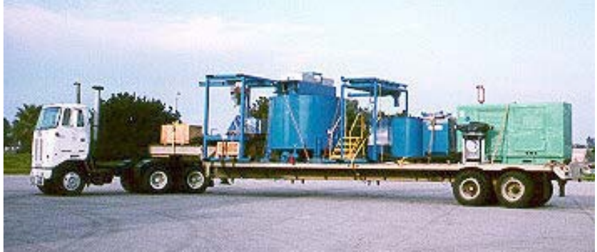
Figure 4—Mixer modules loaded on flat bed trailer for transport from SDTDC to Hemet for testing.
