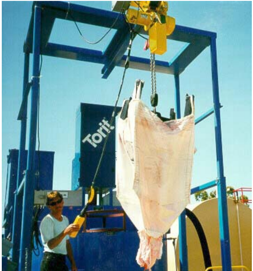
Step 8—Removing empty bag from loading area to ready mixer for next batch. The entire loading process takes less than 5 minutes.
