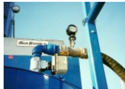
Figure 23—Mixer loading valve assembly.
