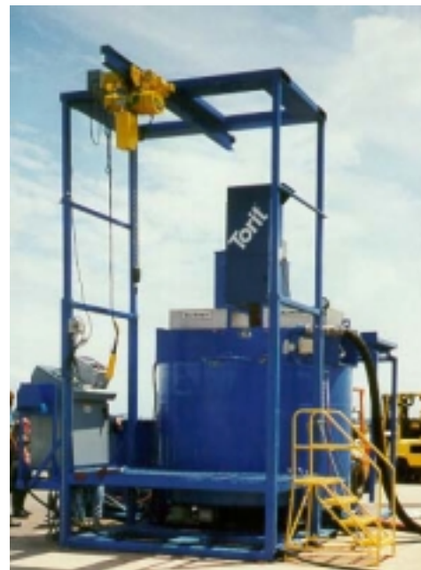
View of Shar Model FSSM-1 with optional loading platform and hoist rack, electric loading hoist & trolley assembly and control panel.
