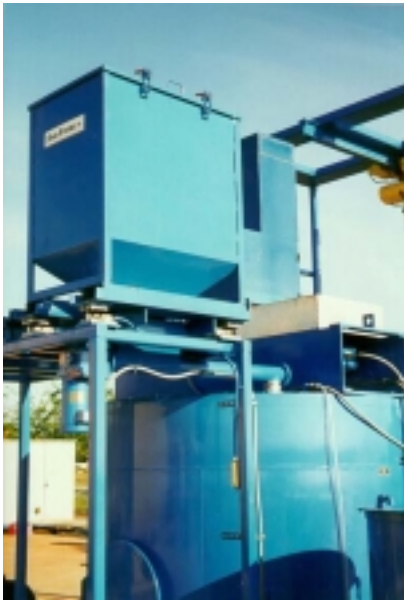
Figure 2—Dry powder feed hopper and conveyor assembly.
