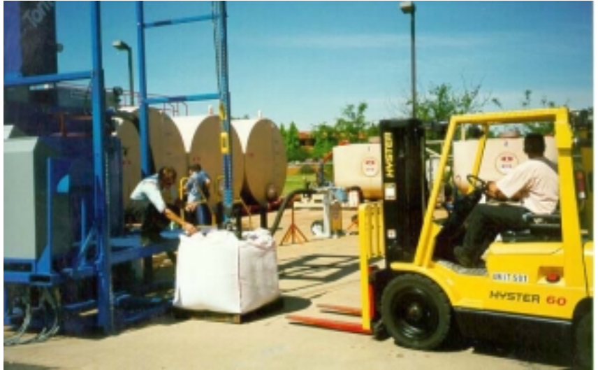
Step 1—Offloading bag from forklift and initial hookup to hoist.
