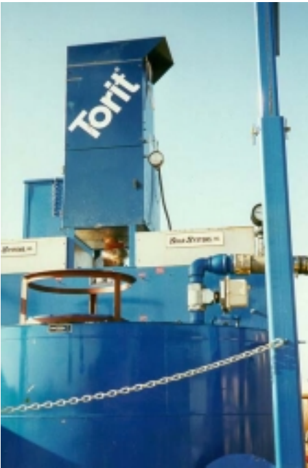
Figure 7—Torit self cleaning dust collector mounted on the top of the mixer.
