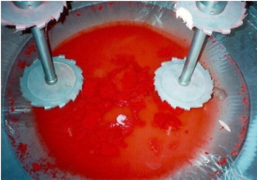
Figure 28—Lumps at the bottom of the mix tank. (View of mixer shafts and turbines.)
