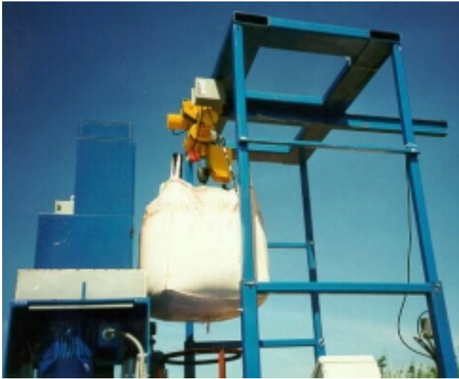
Step 4—Positioning bag over loading hatch safety ring with hoist.
