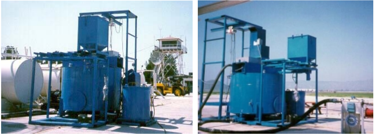
Figure 15—Views of mixer system setup for testing at Hemet-Ryan Airtanker Base.
