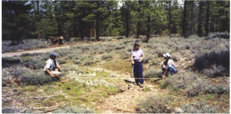
Figure A2. Measuring bankfull channel dimensions on the ephemeral channel upstream of dip.
