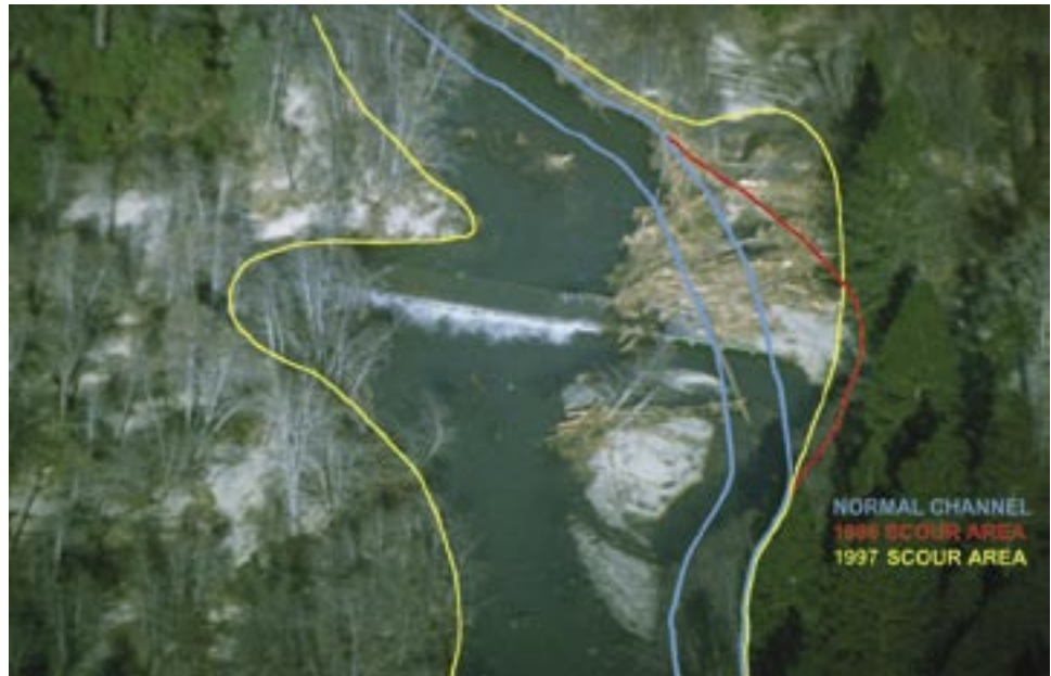
Figure A119. Debris dammed the structure during the 1997 flood event. The main thread of flow shifted to the west and is spilling over the elevated roadway. The white sand deposited everywhere except the higher forested ground in the upper left and lower right of the photo shows that almost the entire area was flooded in 1997. The area that was scoured east of the ford in 1986 is also delineated.
