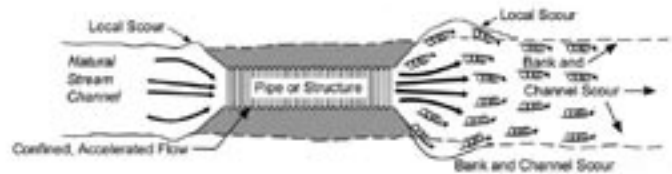
FLOW CONTRACTION THROUGH A STRUCTURE NARROWER THAN THE NATURAL CHANNEL WITH ACCELERATED FLOW AND RESULTING SCOUR AT BOTH THE INLET AND OUTLET
