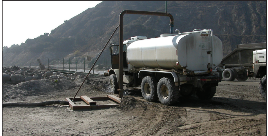
Figure 21—Standpipe used for drafting.
