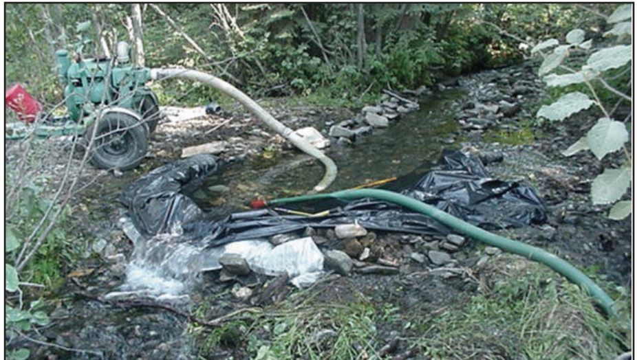
Figure 5—Hard-section hose is commonly used with pumps and water tenders.
