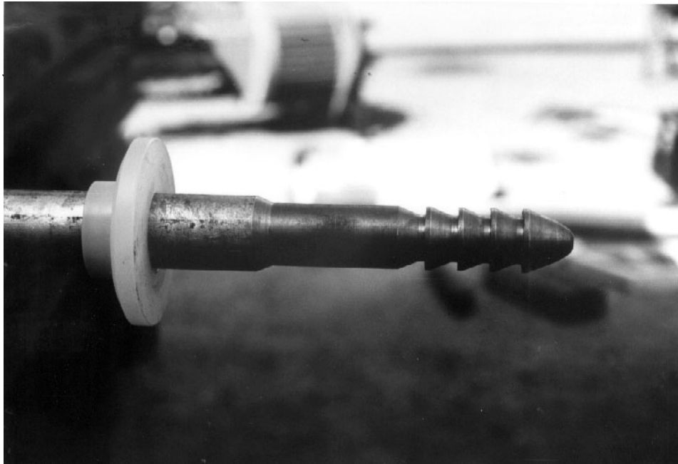
Photo 7. (above) Showing the barbed point of the soil nail for the lead transfer from the collet to the nail.
