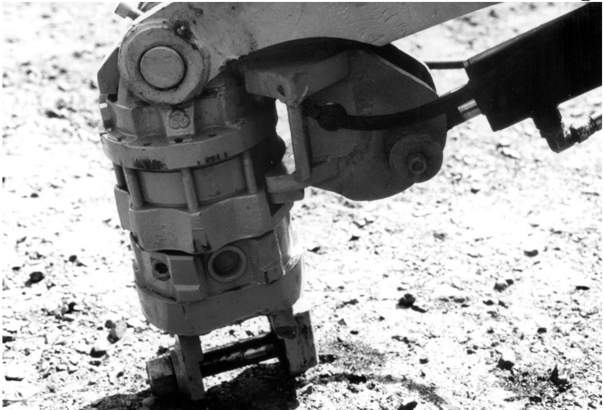
Photo 3. Multiposition hydraulic "knuckle" on the end of the boom for attaching and positioning the launcher.
