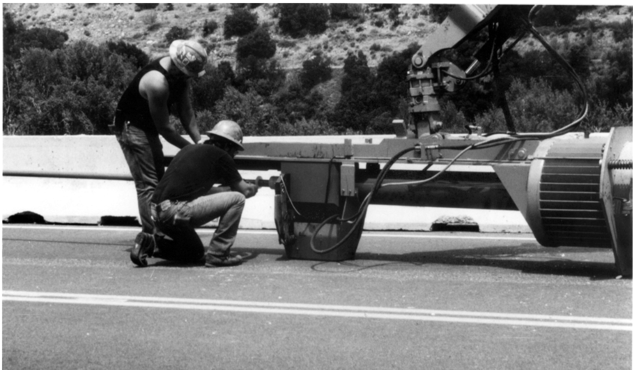
Photo 4. The launcher attached to the hydraulic "knuckle" on the boom and loading a sou nau.
