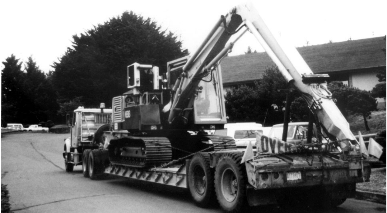
Photo 1. Excavator on transport vehicle. Note the straight boom, the bracket to retain the boom, and the compressor mounted behind the boom.
