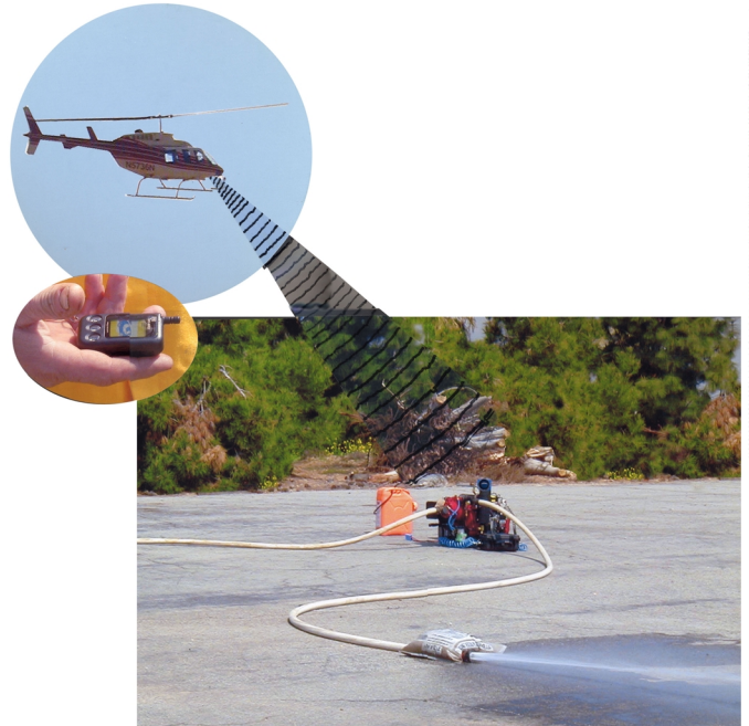
Figure 7—Testing remote pump system from a helicopter.
