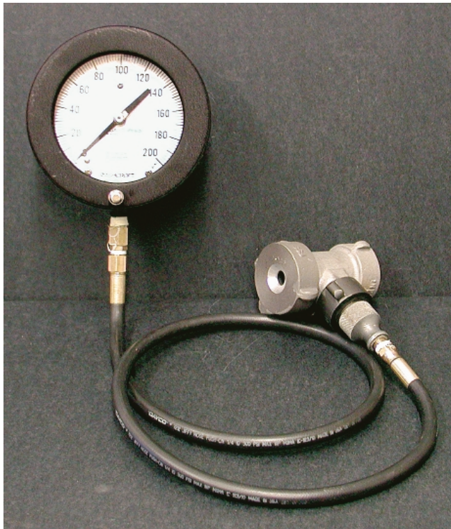
Figure C3 – Photo of square-edged orifice system.
