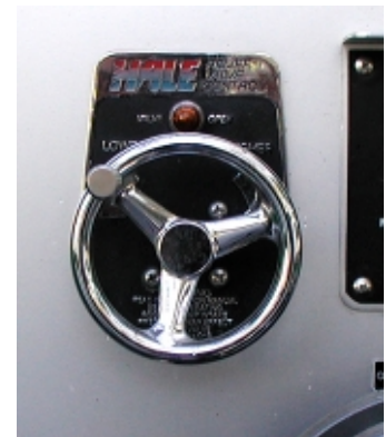
Figure 4—Pressure relief valve control panel.
