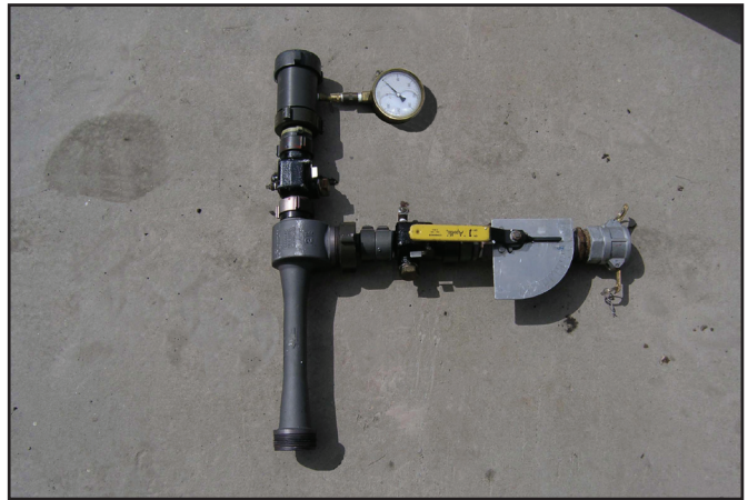
Figure 1—T&D-developed retardant mixer for SEAT bases.
