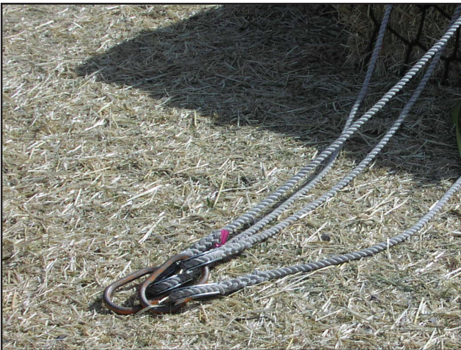
Figure 4—Rodeo method, net ready for hook up. The retrieval line attaches to cage of remote hook and rings on net attach directly into remote hook.
