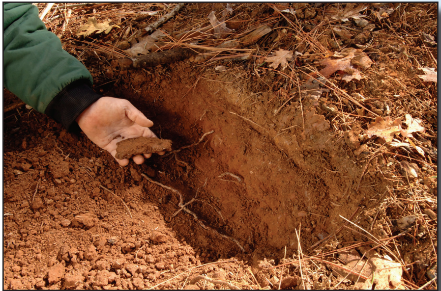
Figure 2-19—Compaction moderate. Increased resistance is evident to approximately 8 inches.
