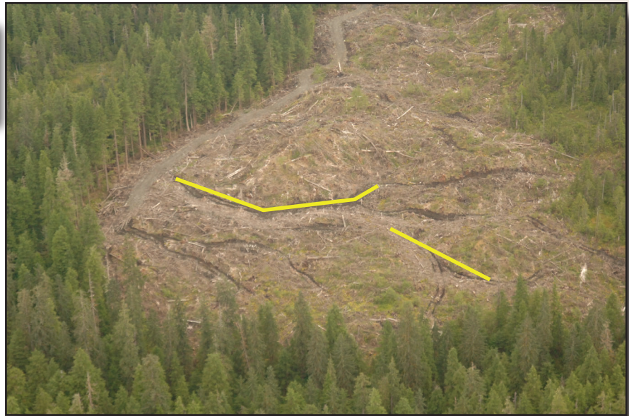
Figure 6-4—Vegetation: Sitka spruce and western hemlock. The surface soil texture is gravelly silt loam. Private timber lands are at high risk to mechanical-equipment impacts due to low load-bearing capacity of the soil. In remote areas aerial reconnaissance may help identify areas of concern. Ecomap Section M245C - Southern Alexander Archipelago, Alaska Region.
