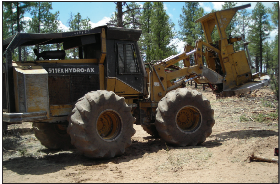
Figure 7-9—Often a larger feller-buncher will work with the smaller, three-wheeled feller-buncher to fell the large-diameter trees in a treatment unit.
