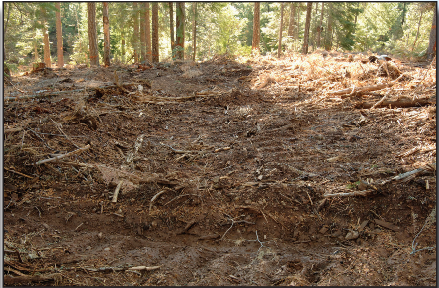
Figure 2-27—Soil-disturbance class 2, wheel tracks are evident, forest-floor layers are missing, soil-displacement is evident, and soil compaction is increased (up to 12 inches).
