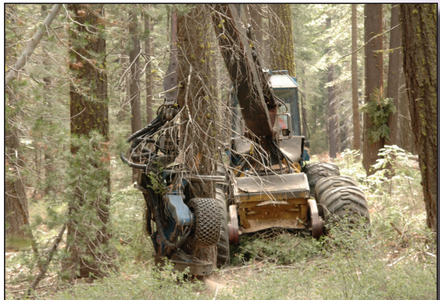
Figure 7-4—A harvester equipped with a processing head felling a tree.
