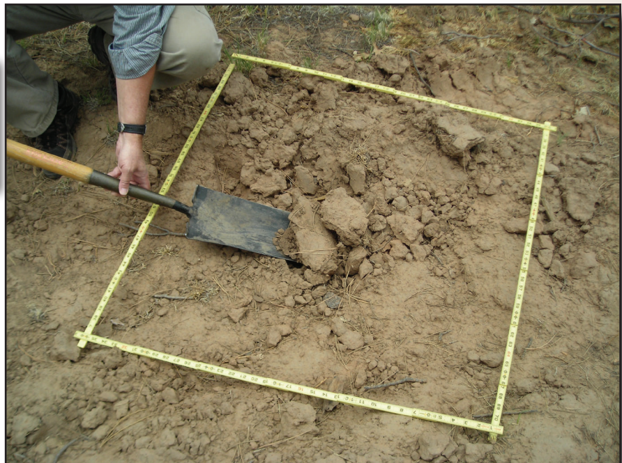
Figure 6-17—Vegetation: Ponderosa pine, white fir, Douglas-fir, and some areas of pinyon pine and juniper. Rutted segment of skid trail has deep compaction and platy soil structure without roots (photo March 2007). Ecomap Section M313A - White Mountain-San Francisco Peaks-Mogollon Rim, Apache-Sitgreaves National Forest, Southwestern Region.
