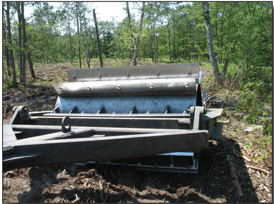
Figure 7-26—A roller-chopper drum with blades designed to “chop” downed material.
