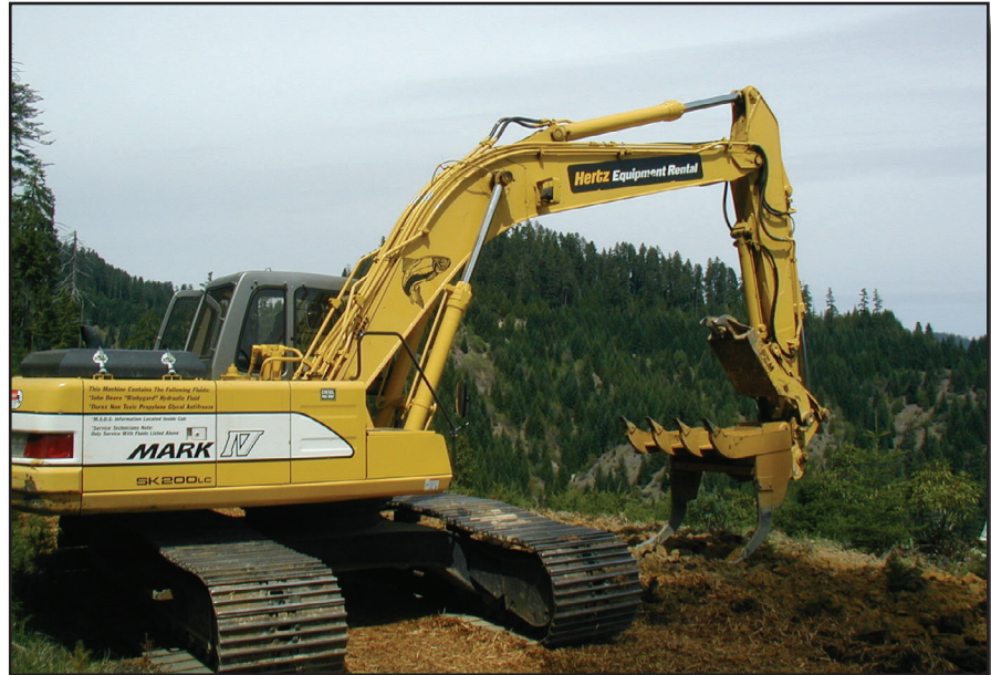
Figure 7-29—A modified excavator head to decompact landings and skid trails.
