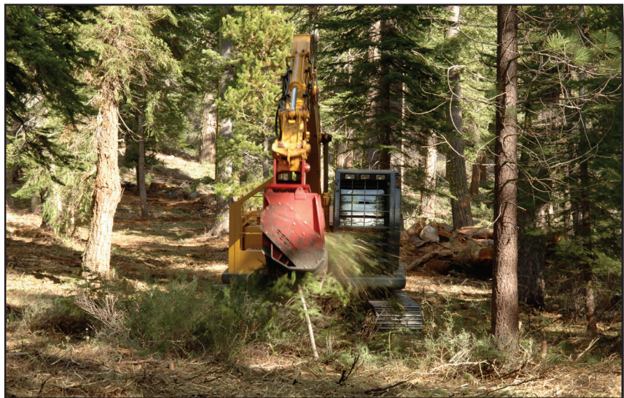
Figure 7-23—An excavator with a masticator attachment is shredding live vegetation.
