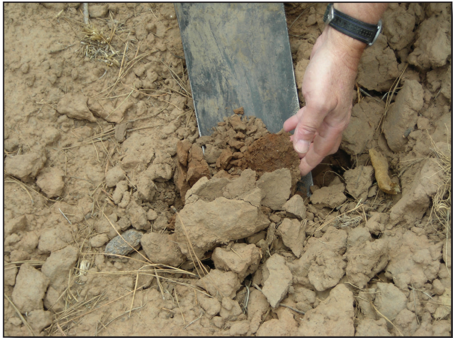
Figure 6-18—Deeply compacted soils can be difficult to sample.
