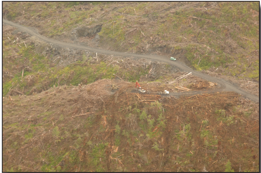
Figure 7-20—Logs are brought up to the landing area with the small swing-yarder and then sorted and loaded onto log trucks.
