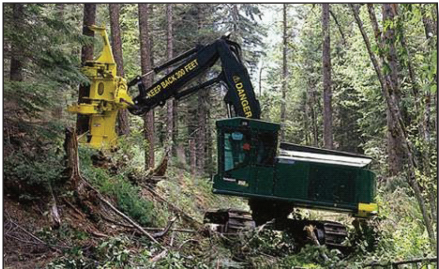
Figure 7-2—A tracked feller-buncher working at a single location. Once all trees are felled and bunched at this location, the machine will move to the next setting.
