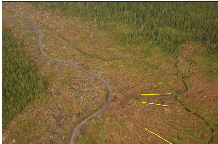
Figure 6-5—Extensive rutting can occur without slash mats to protect the soil.
