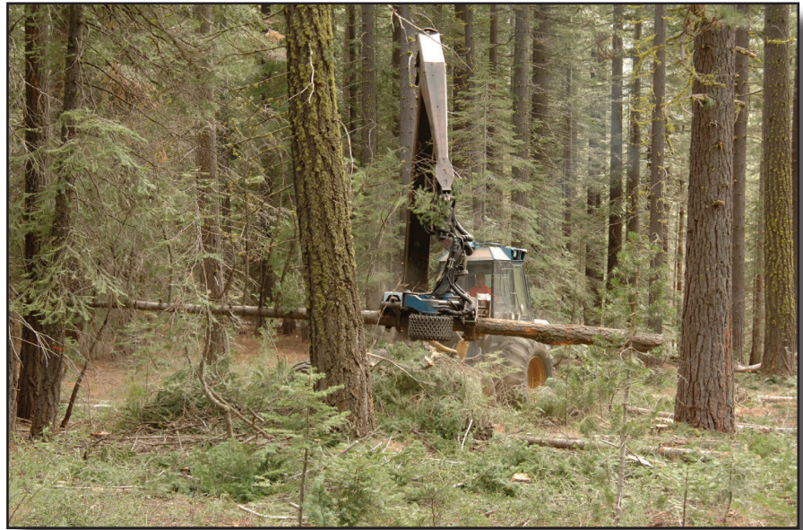
Figure 7-5—A processing head is delimbing the tree prior to its being cut into lengths and picked up by a forwarder.
