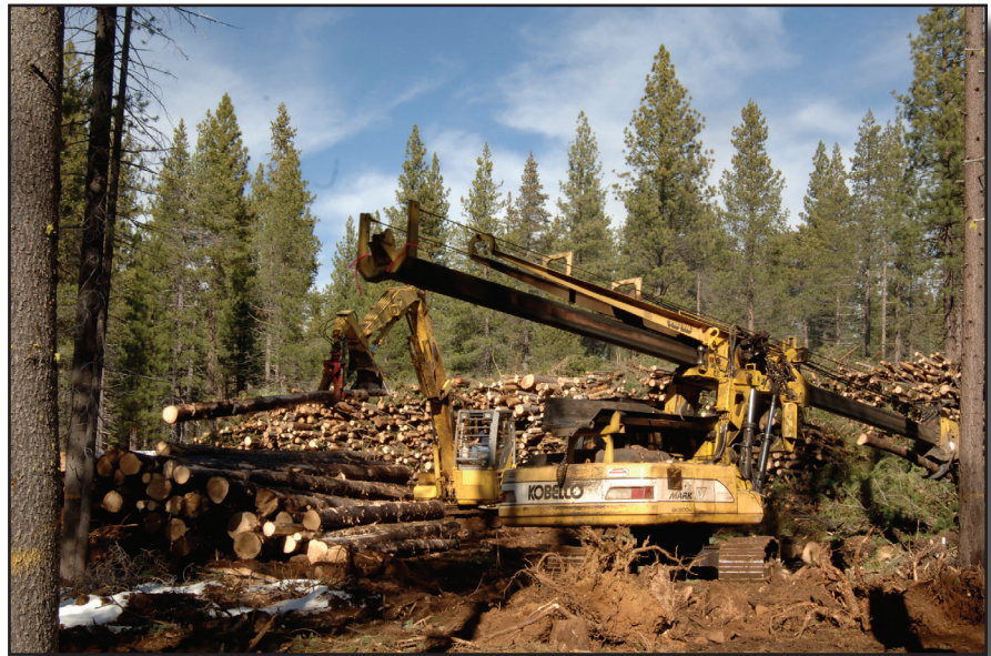
Figure 7-16—Logs are delimbed, cut, and sorted prior to being trucked to the sawmill or cogeneration power plant. The landing size is an important consideration from both a safety and a soil-impact perspective.
