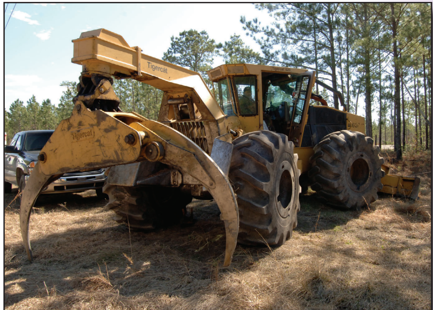
Figure 7-11—This large grapple-skidder can bring a large load of trees into a landing area. Identify compaction or rutting concerns in areas with high risk-rated soils.
