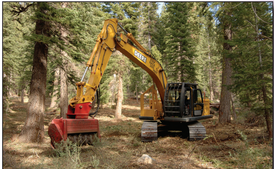
Figure 7-24—The masticator-head grinds or flails woody vegetation into chips that provide soil cover.
