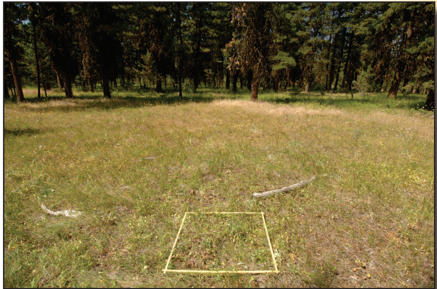
Figure 4-32—Vegetation: Mixed conifer forest. Soils in this area are influenced by a mantle of volcanic ash from Mount Mazama. The surface soil texture is silt loam. The photograph illustrates legacy disturbance from a timber harvest approximately 20 years ago. Visual indicators of class-1 disturbance in previously harvested units include vegetation composition and vigor, depth of forest floor, presence of stumps or cull decks, increased resistance to penetration with tile spade, and or platy soils. Ecomap Section M332G - Blue Mountains, Umatilla National Forest, Pacific Northwest Region.
