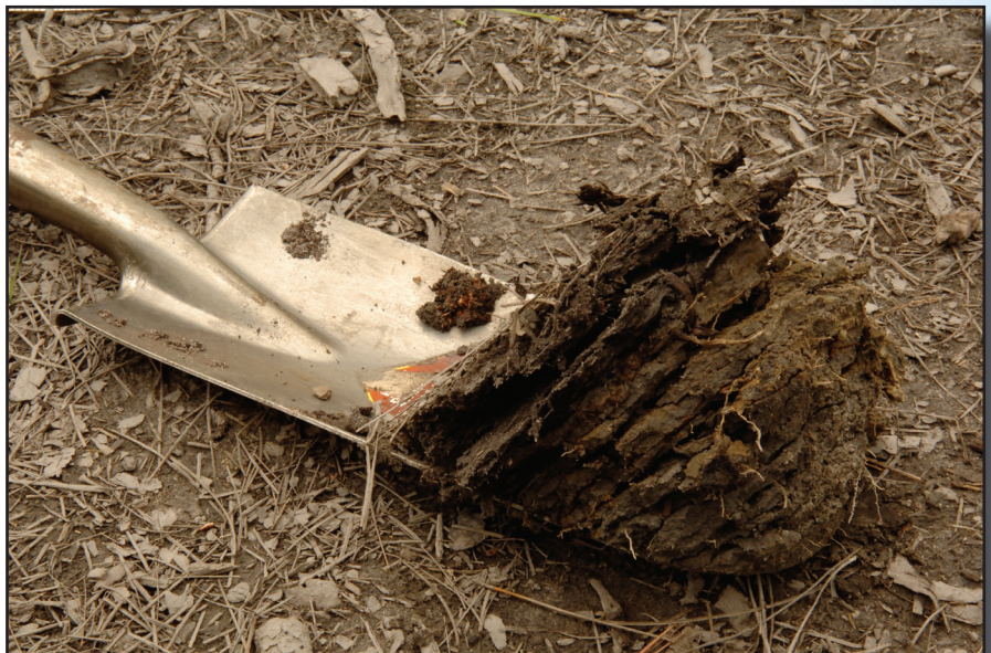
Figure 2-24—Deep platy structure is evident in the main skid trail.
