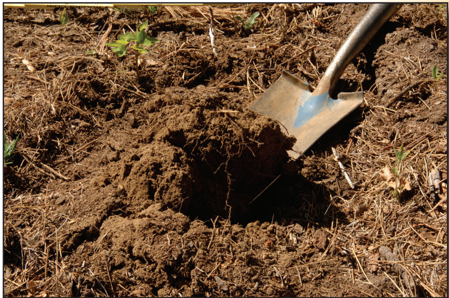
Figure 4-13—Closeup of the soil structure from the skid trail in figure 4-12, showing no signs of increased compaction.
