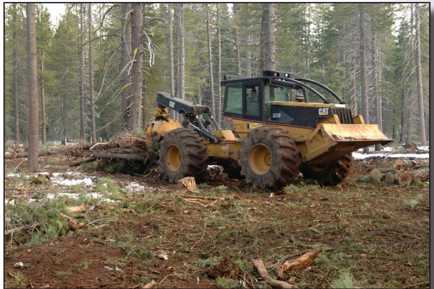
Figure 7-15—The bundle of trees is pulled into the landing area for further processing.
