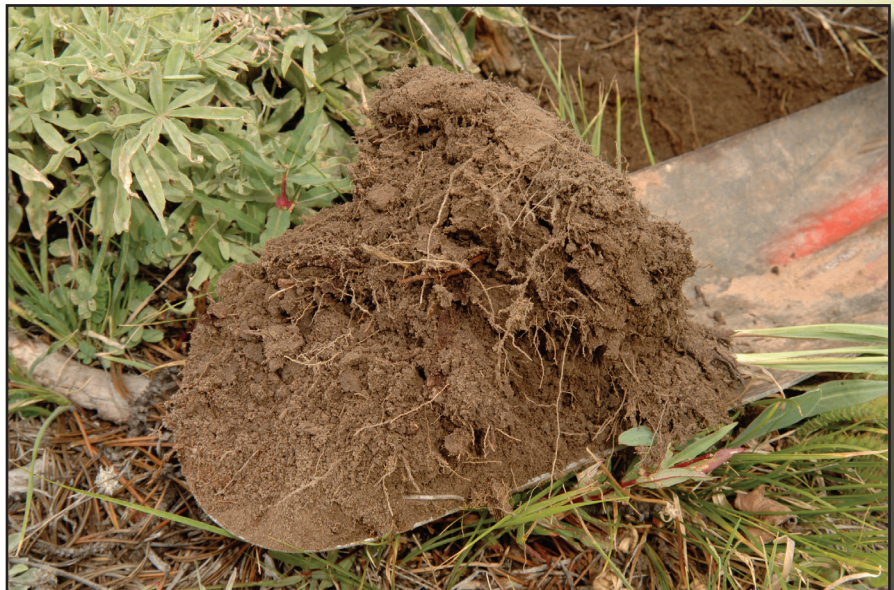
Figure 3-12—Close-up of the soil structure from this undisturbed area in figure 3-11. Notice the abundance of roots throughout the sample.
