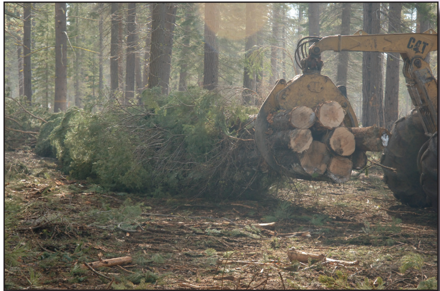
Figure 7-14—The grapple-skidder moves into position and grabs an entire bundle of trees.
