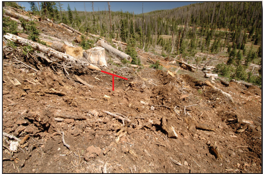
Figure 6-16—Vegetation: Western spruce-fir forest. The surface soil texture is loam. This unit is part of an insect-salvage harvest of Engelmann spruce. Deep ruts and surface soil displacement from turning equipment reflect a class-3 soil disturbance. The soil scientist reviewed the area to explore options for yarding the cut trees to reduce and ameliorate effects to soils. Steep slopes add to the challenge of removing insect-salvage trees from the site. Ecomap Section M341C - Utah High Plateaus and Mountains, Dixie National Forest, Intermountain Region.
