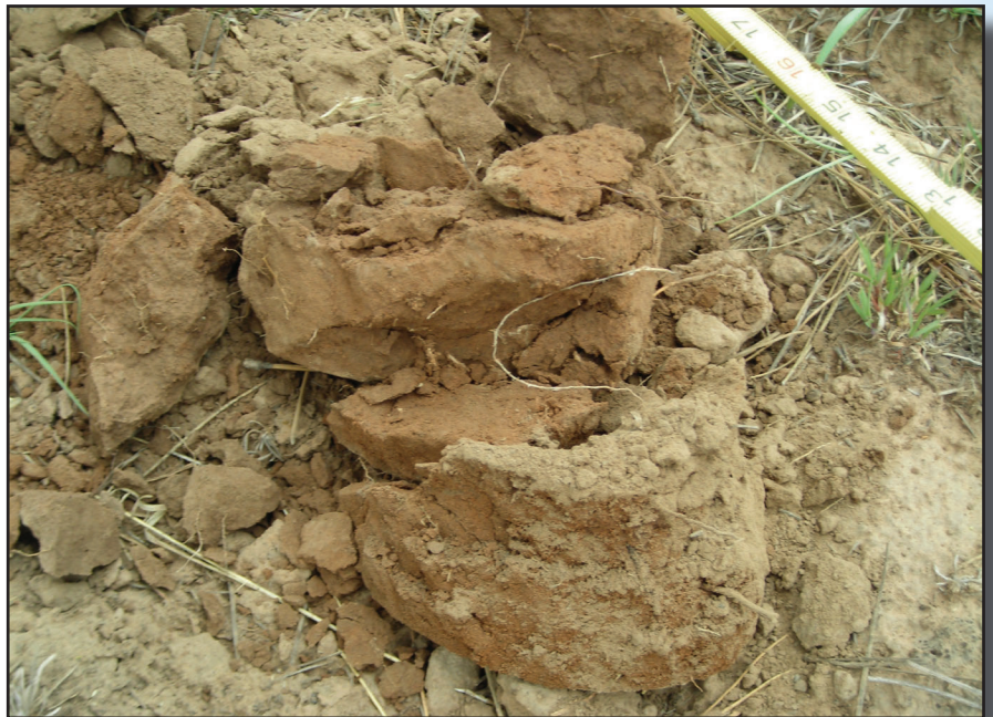
Figure 2-20—Compaction deep. Increased resistance is greater than 12 inches in depth on this main skid trail.
