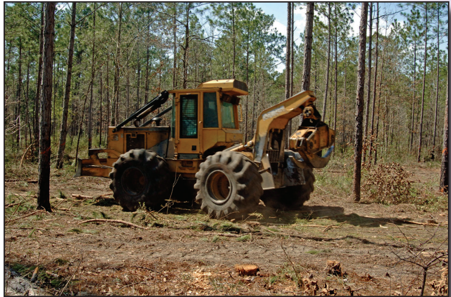
Figure 7-10—A small grapple-skidder can maneuver easily in tight areas.
