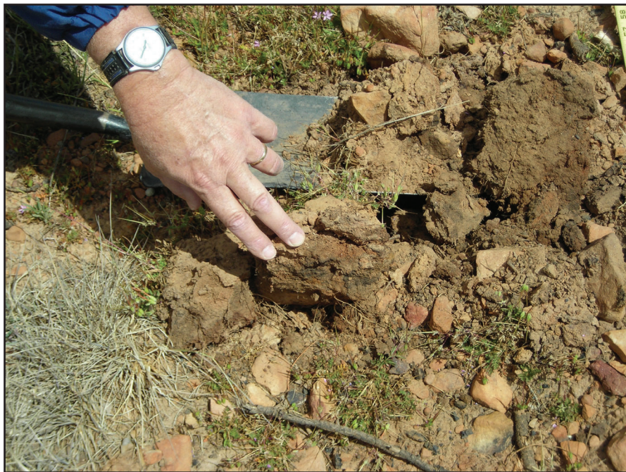
Figure 2-18—Compaction shallow. Increased resistance and compression is evident but the rocky soils ameliorate the depth and severity of compaction.
