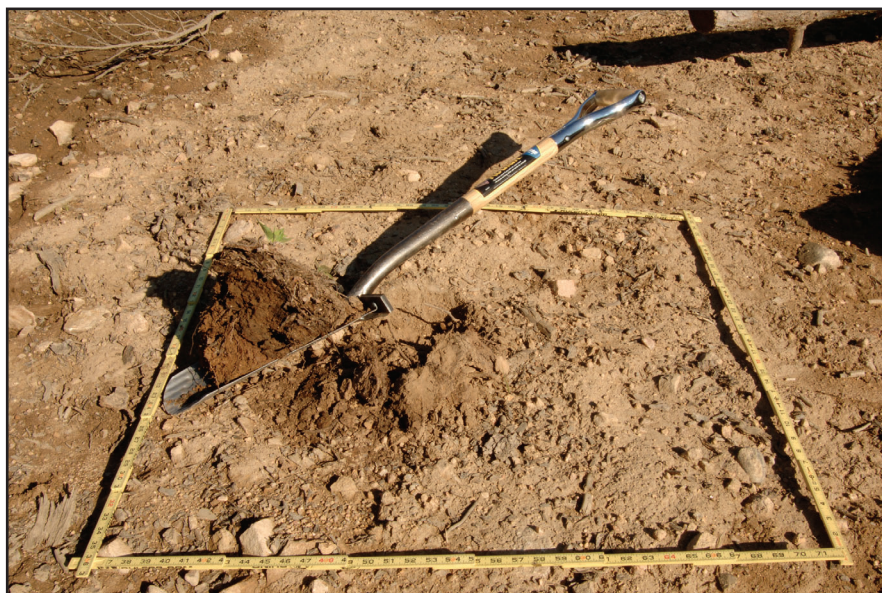
Figure 6-22—Closeup of soil compaction within the skid trail.
