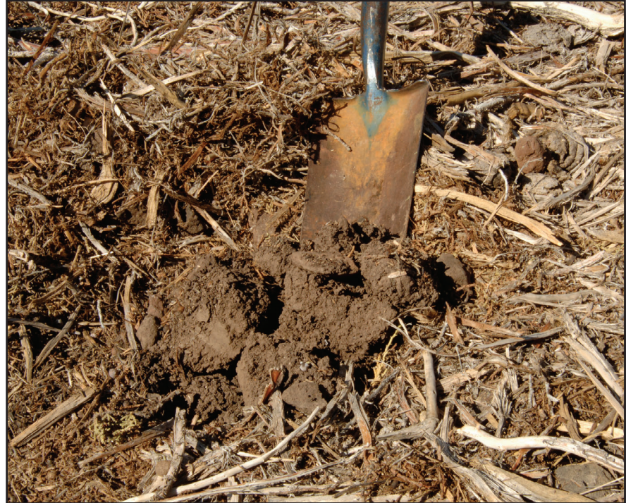
Figure 4-19—It is important to dig into the soil profile to check for signs of increased resistance and depth of soil compaction.
