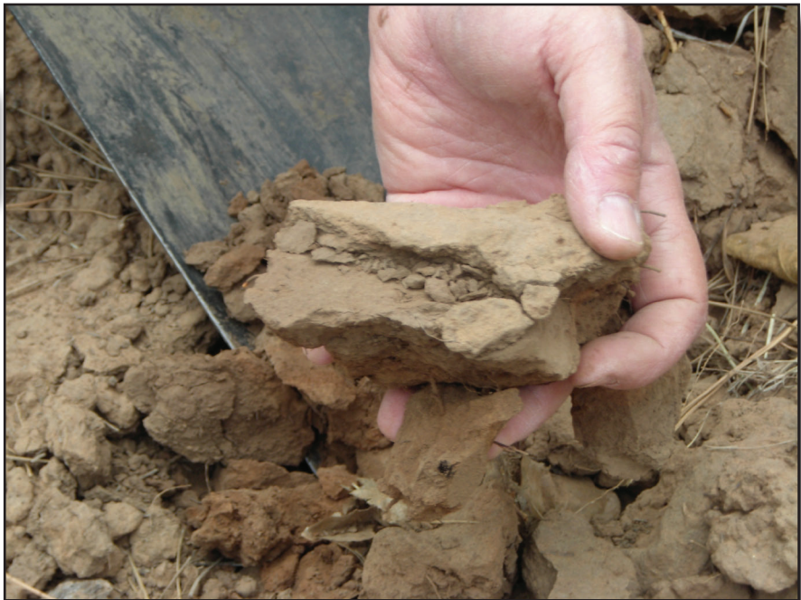
Figure 6-19—Compacted soil from main skid trail that may have been used during suboptimal moisture conditions.
