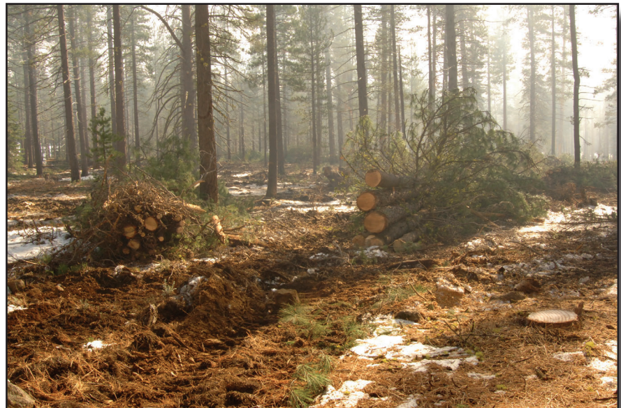
Figure 7-13—Bundles of trees are ready to be moved into the landing area for sorting and processing.
