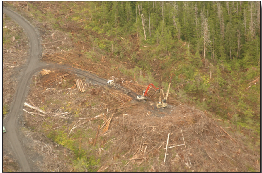
Figure 7-19—A cable-yarding operation is set up on a spur road harvesting trees on this steep slope.
