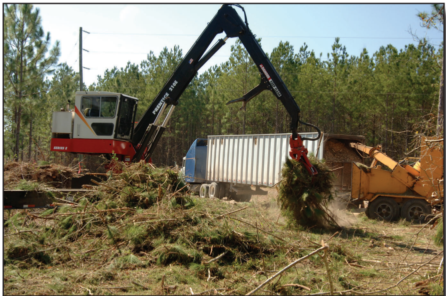
Figure 7-17—At the landing site some of the logs and residues may be processed further. A chipper is often brought into the landing once all the saw-logs are removed. Small-diameter logs may be chipped. Limbs and branches may be redistributed on skid trails or placed in a pile for burning.
