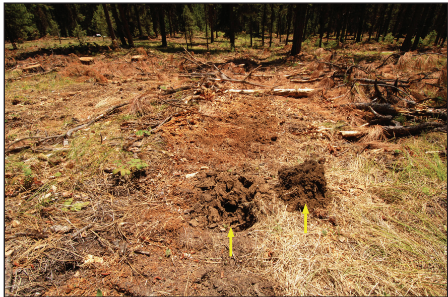
Figure 4-31—When conducting an assessment, compare the soil within the track and undisturbed area to assess the soil compaction.
