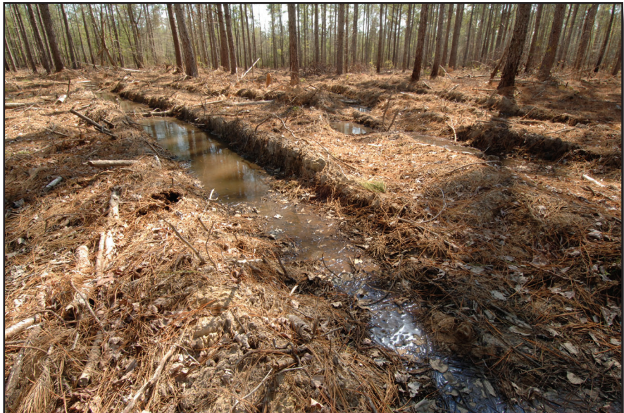
Figure 2-14—Deep ruts formed in soils with a high water table.
