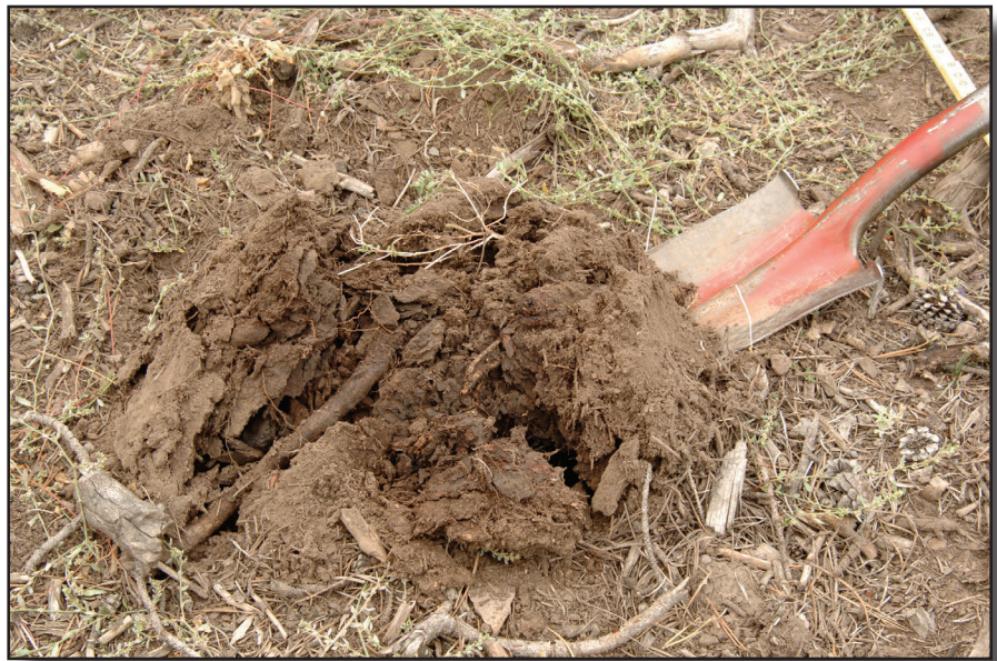
Figure 5-22—A closeup of the skid trail illustrates weak platy soil structure.
