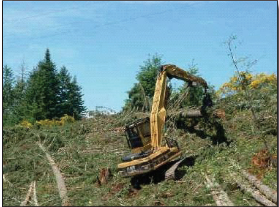
Figure 7-21—Working on the sideslope, the shovel-yarder is moving the logs towards the landing.
