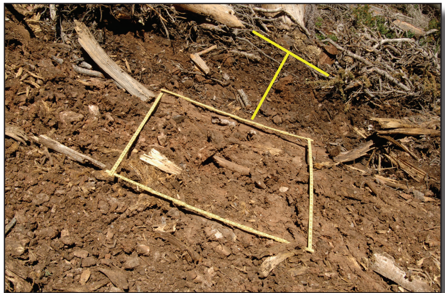
Figure 6-15—Deep ruts and displaced soil from turning equipment is evident.
