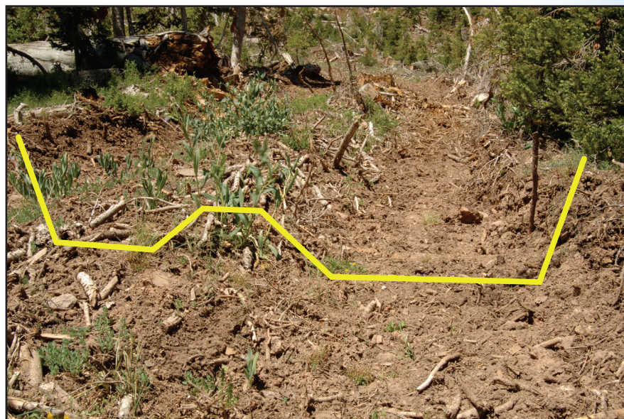
Figure 2-12—Moderate rutting on the skid trail, during suboptimal moisture conditions.
