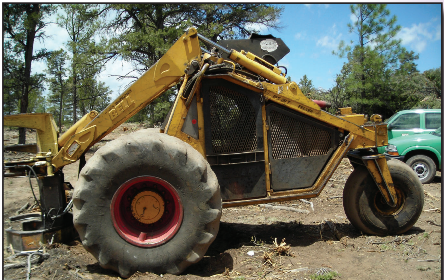
Figure 7-8—Fast and maneuverable, the three-wheeled feller-buncher can fell small-diameter trees quickly.
