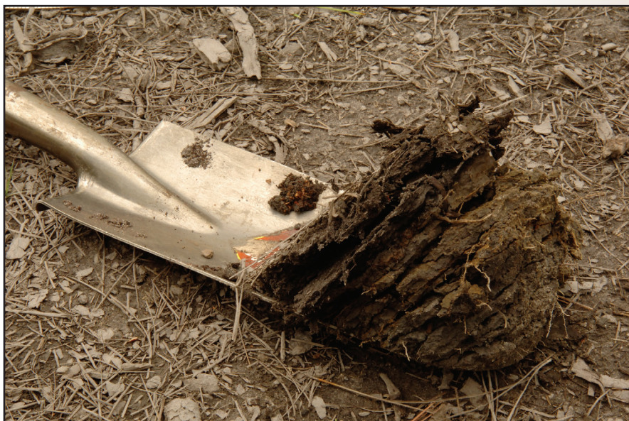
Figure 6-8—Closeup of platy soil structure from the main skid trail. Notice that there are few roots within the soil.
