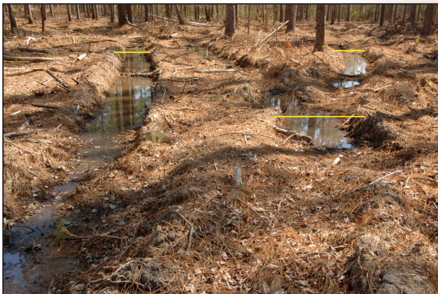
Figure 6-9—The soil risk rating for this area would identify the low load-bearing capacity of these soils due to a high water table. Deep ruts were created with a single equipment pass. Ecomap Section 232C - Atlantic Coastal Flatlands, Francis Marion and Sumter National Forest, Southern Region.
