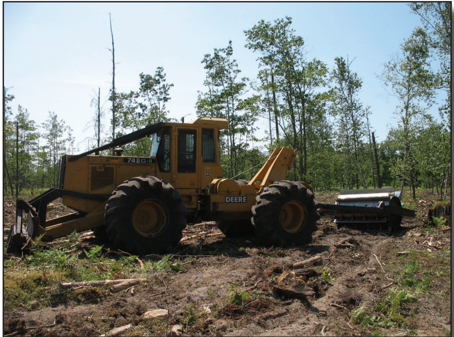
Figure 7-27—A roller-chopper is breaking up forest residues on the Hiawatha National Forest after a salvage harvest.
