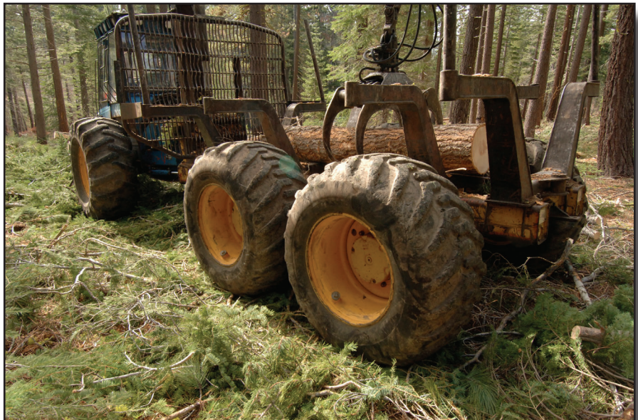
Figure 7-6—A forwarder loading processed logs into the bunk. Note use of the slash mat that was created to reduce soil disturbance.
