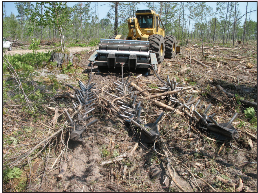
Figure 7-28—Chains have been attached to create openings and expose bare soil.
