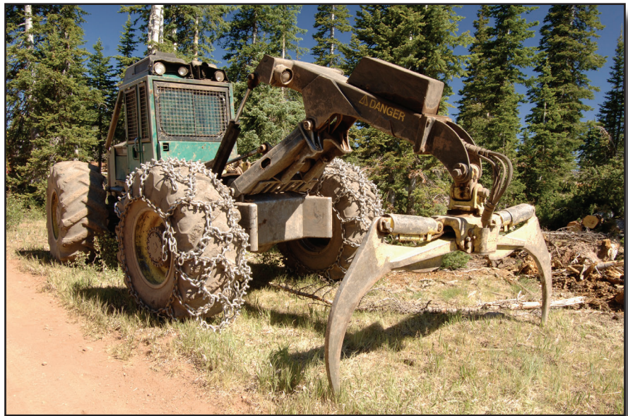
Figure 7-12—A grapple-skidder with chains used for winter logging operations.
