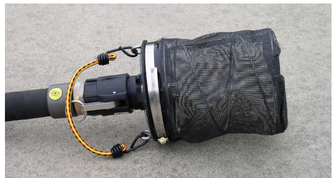
Figure 2. Hose-end fish strainer for drafting operations.
