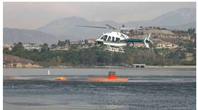
Figure 1. Light helicopter dipping from fish strainer with a 180-gallon Bambi Bucket.
