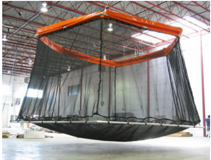
Figure 3. View of fish strainer suspended in air.
