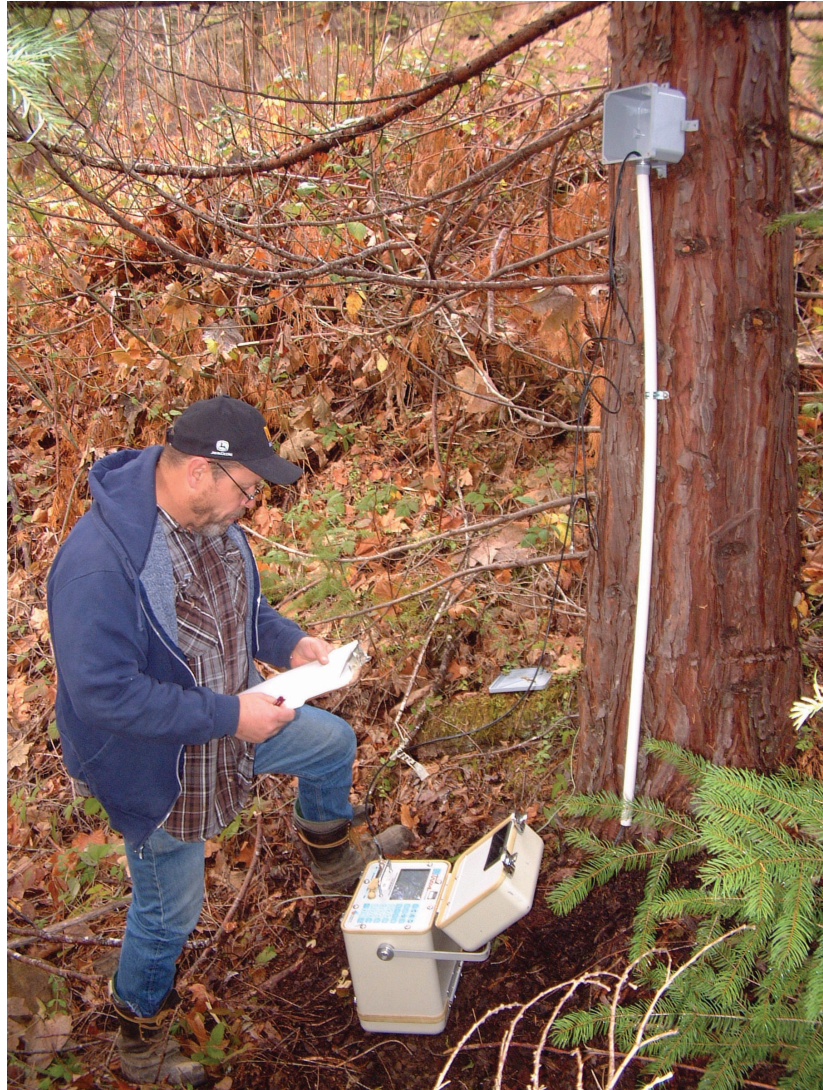
Figure 3—Reading the TDR cables.
