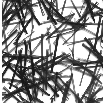
Figure 3.2a— Reinforcing fibers. (Tammy Stewart, geosyntheticssolution.com)
