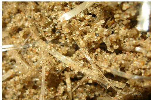
Figure 3.2—Discrete reinforcing fibers.
