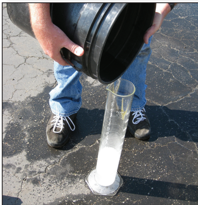
Figures 2a and 2b—Collecting and measuring volumes of water from the leak.
