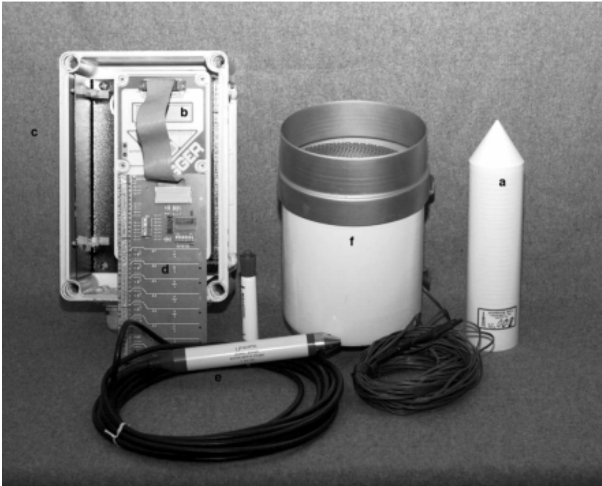
Figure 3—Equipment used for monitoring the effects of roads on groundwater piezometric surfaces. (a) PVC well tip. (b) Unidata Starlogger. (c) Weatherproof enclosure. (d) Field termination strip. (e) Hydrostatic pressure transducer. (f) Tipping bucket rain gage.
