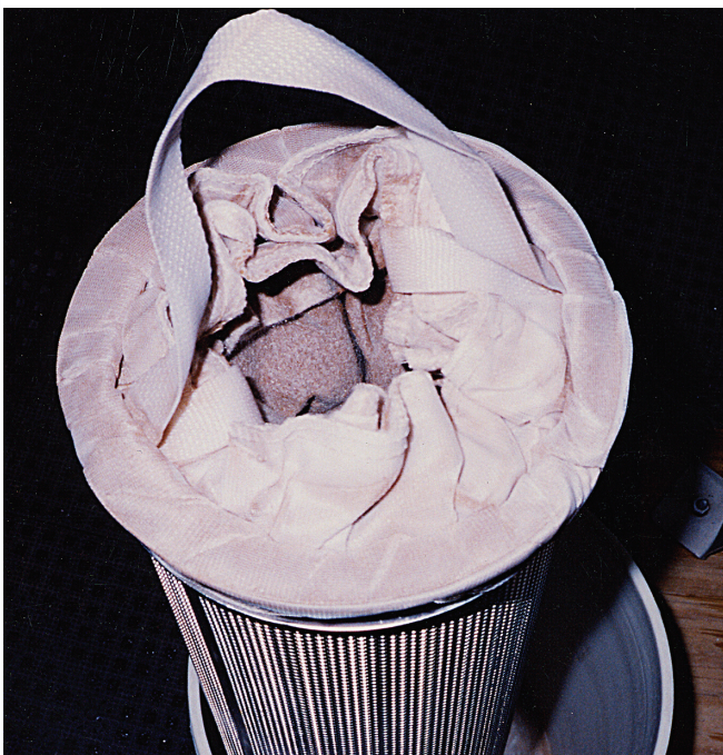
Figure 76—Used bag filter in support basket.
