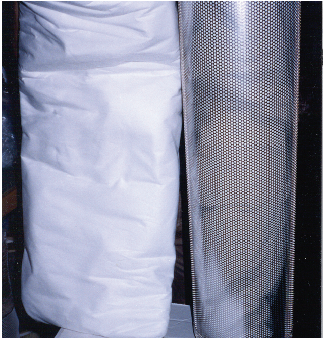
Figure 75—New bag and support basket.
