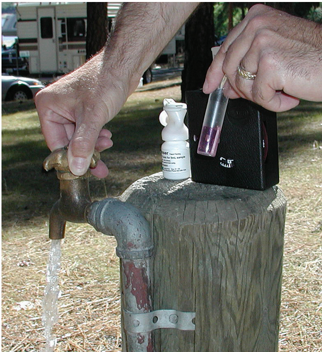
Figure 80—Chlorine residual test.
