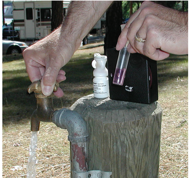
Figure 54—Test water for free chlorine.
