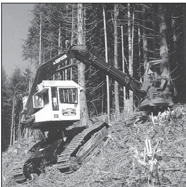
Figure 10—Timbco T445C feller-buncher with the Quadco 22-inch disk saw.
