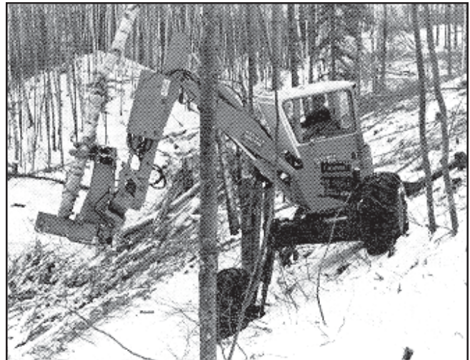
Figure 14—The Menzi Muck with a feller-buncher head is one of few machines that can operate brush cutters on slopes greater than 50%. They are cost prohibitive to run and are not readily available. ☹️
