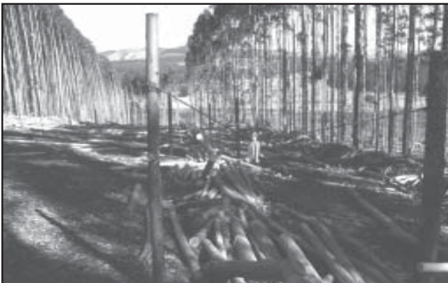
Figure 13—Eucalyptus clearfell harvesting with Howe-Line monocable system. (Photo courtesy of Professor Loren Kellogg, Oregon State University.)
