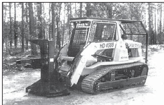
Figure 9—The ASV Posi-Track is a smaller, rubber-tired machine that shows good stability on slopes.
