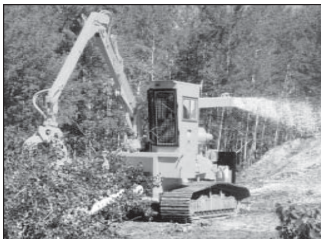
Figure 8—Track Bandit Model 1900 self-propelled whole-tree chipper.
