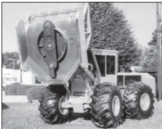
Figure 3—The cutting head on the Kendall Cutter is a typical vertical shaft with free-swinging cutters.
