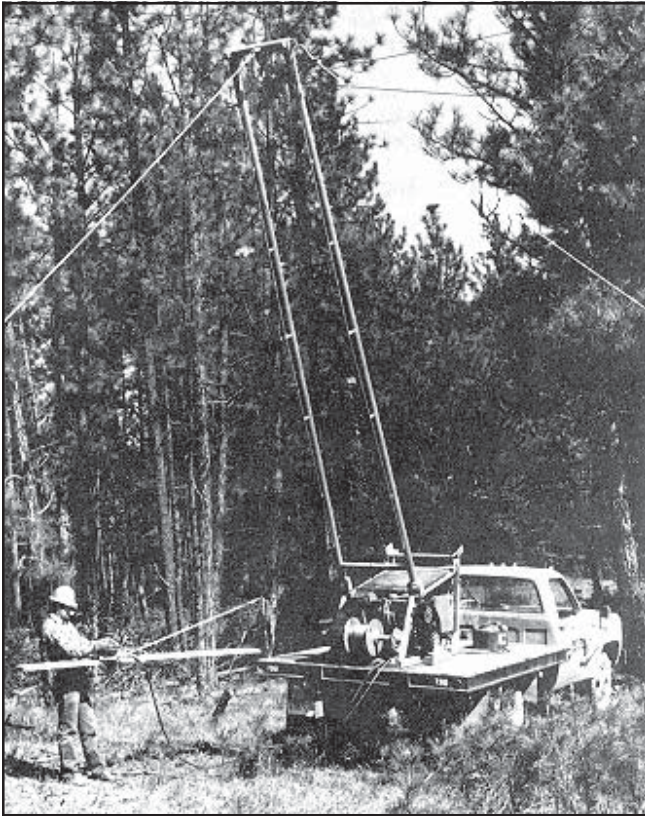
Figure 12—The Bitterroot Miniyarder would be suitable for yarding smaller wood.
