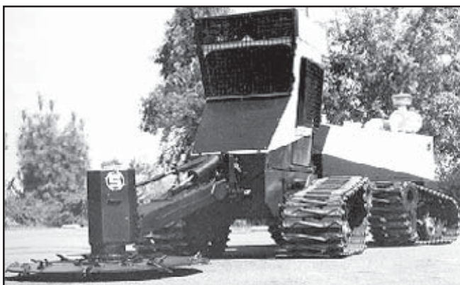
Figure 6—The Shar 20 has a vertical shaft and a fixed-tooth disk.
