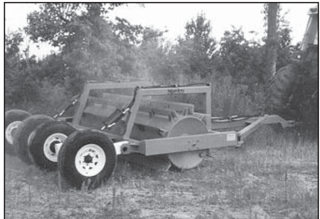
Figure 2—Rolling chopper used for land clearing.
