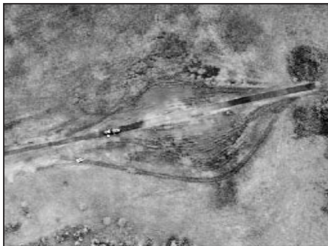
Figure 8—This aerial image shows a recently installed section of hardened trail crossing a wetland in southcentral Alaska. The new trail alignment defines a single route of travel that will prevent the continued development of braided trails.
