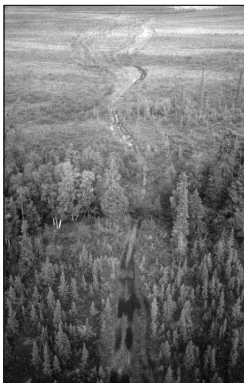
Figure 7—A heavily used OHV trail in Alaska crosses two distinct soil types. In the foreground, the trail passes through a mixed forest ecosystem where the soils support use along a single track. In the background, the trail crosses degraded wetland soils where users have created a braided trail. Managers should consider rerouting the trail to stay within the forest system.
