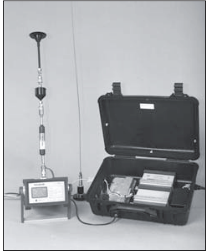
Figure 6—DataRAM connected to the telemetry unit.
