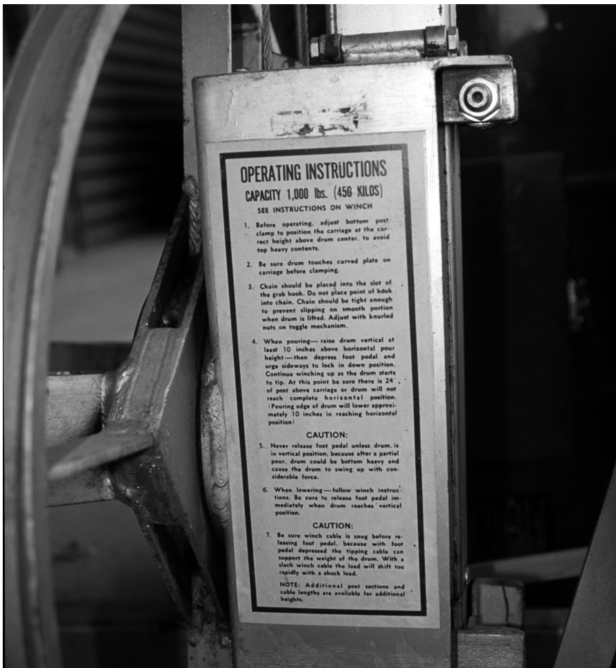
Figure 1—Cranes and hoists should be properly marked with pertinent safety information and load limits.
