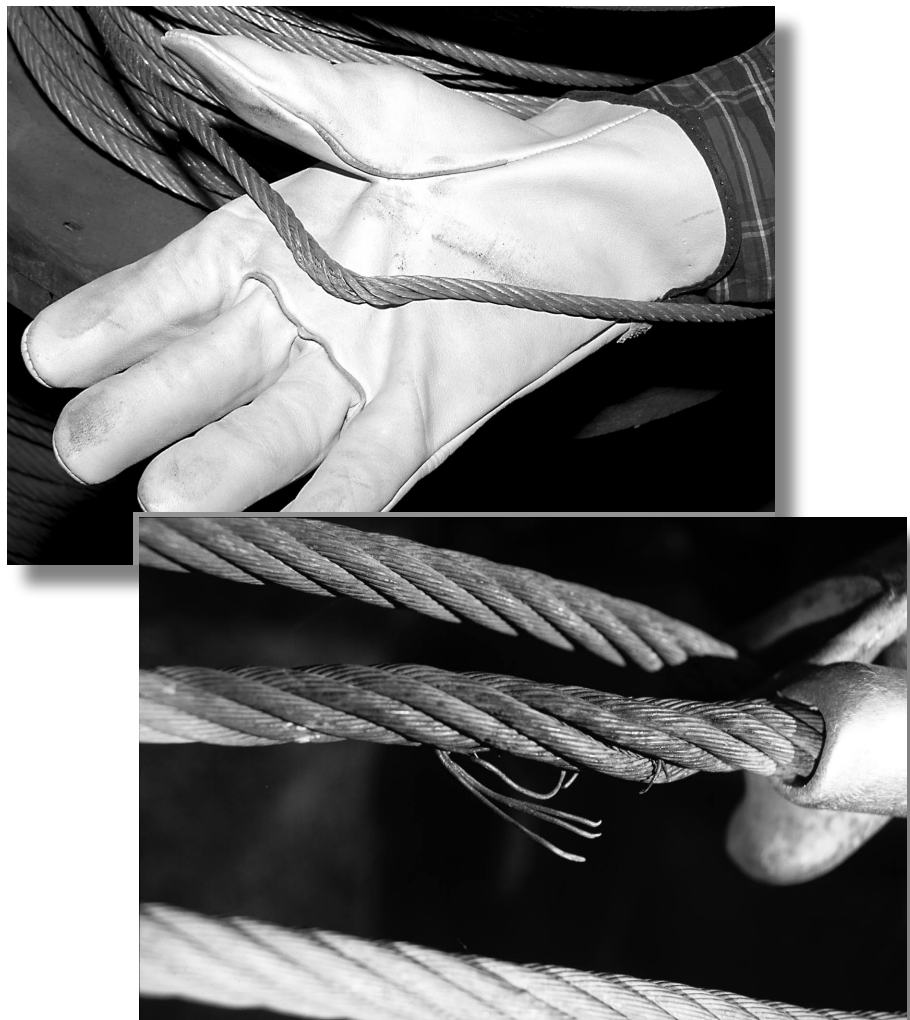
Figure 3—Inspect wire rope for crushed areas or broken wires.
