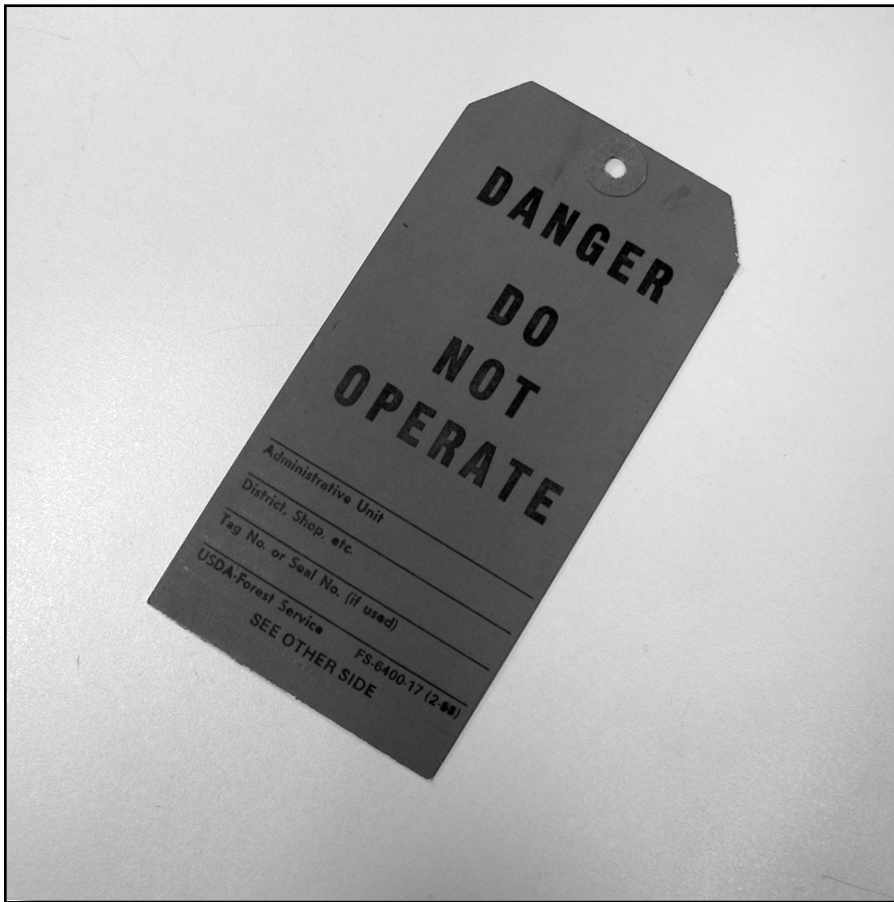
Figure 4—Mark unsafe or damaged equipment with a “red tag” (FS-6400-17) and remove it from use until it has been repaired.
