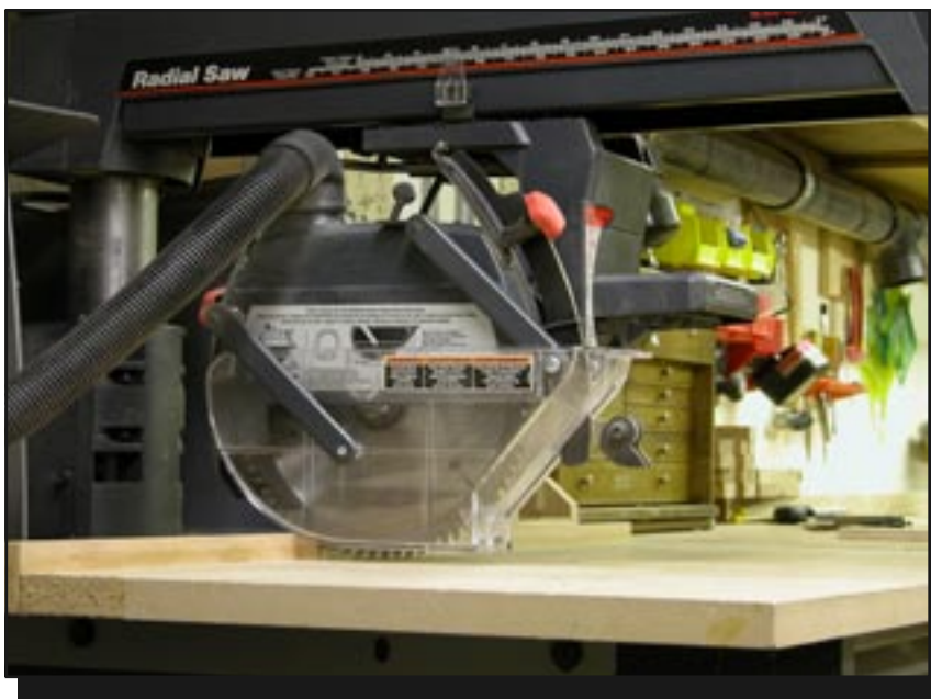
Figure 10—Proper guards and shields on equipment and machinery are important safety devices that may be noticed during facilities condition assessment surveys. Although this sort of safety hazard is not technically part of a condition survey, missing guards and shields should be brought to management's attention so the problem can be corrected immediately.
