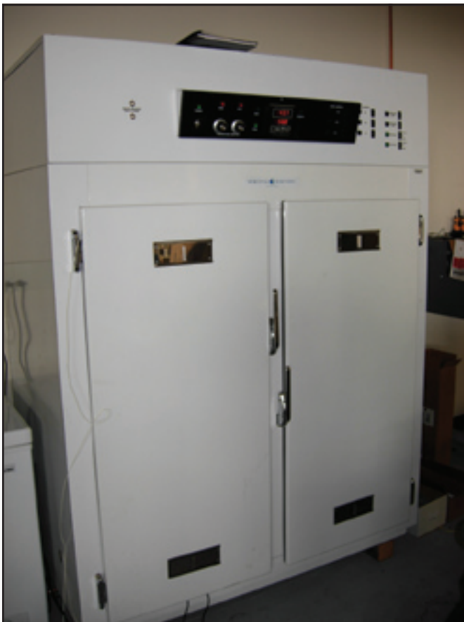
Figure B-1—An environmental chamber was used to conduct the extreme hot temperature startup and operation tests.
