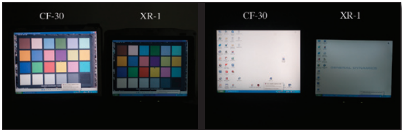
Figure I-2—The laptops screens were also compared in the dark. It is important to law enforcement officers that the screen is not bright enough to compromise their position in the dark. The XR-1 screen was much darker at its lowest setting, but was still readable.
