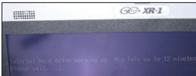
Figure A-3—Neither laptop started immediately. They displayed a screen like this one (XR-1 laptop) stating it would take time for the laptop to warm up. Both started within 5 minutes.
