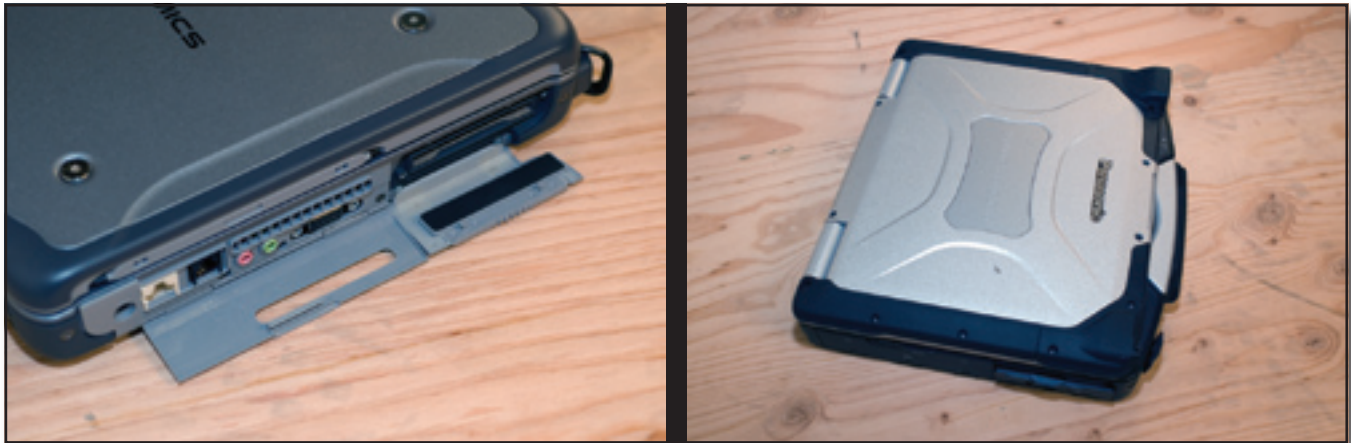
Figure D-2—The covers to drives and ports came open on most of the drops on the XR-1 laptop. This could pose a problem if the laptop were dropped near water or mud. One cover came open of the first drop on the CF-30 laptop. It is unsure if this cover was fully latched before the drop. It did not open on any subsequent drops.
