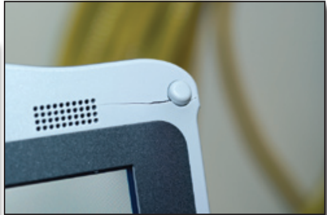
Figure 3—The laptops were drop tested to test shock resistance. The laptops were dropped onto plywood from 3 feet on all six axes. The XR-1 laptop developed a crack in the case around the screen after one of the drops.
