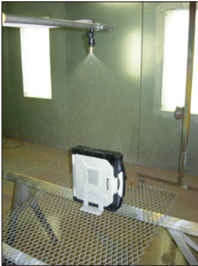
Figure C-3—The laptops were placed on a metal grate and held upright using bookends.
