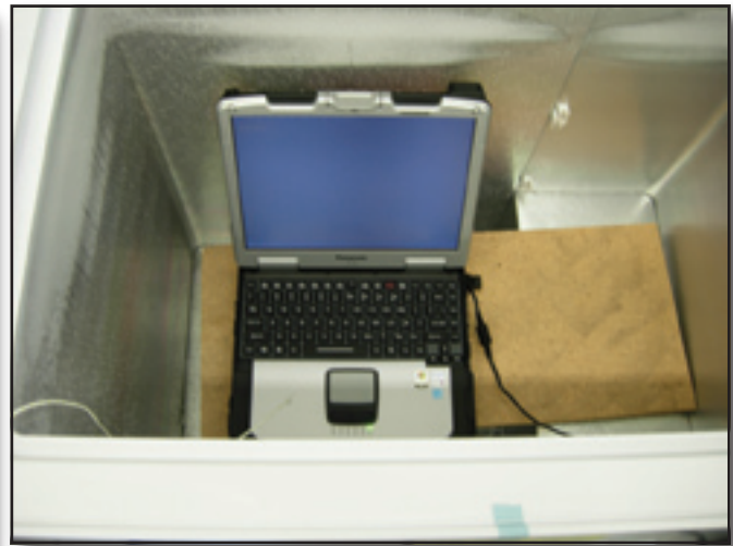
Figure A-2—Each laptop was placed in the freezer. The laptops were left in the freezer for 2 hours once they reached a temperature of -15 °F. Then they were started.
