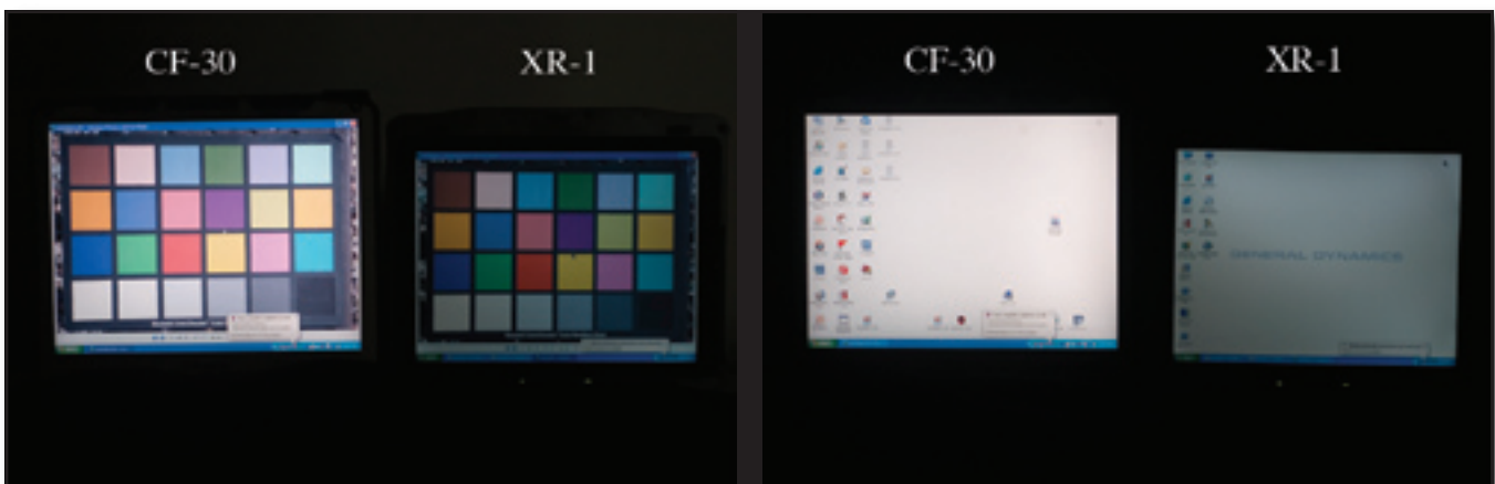
Figure 5—The laptops' screens were also compared in a dark setting. It is important to law enforcement officers that the screen is not too bright in the dark so their position is not compromised. The XR-1 screen (the right screen in each pair of photos) was much darker (but readable) at its lowest setting.
