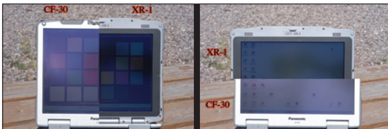
Figure I-1—The laptops were compared side-by-side to determine how well the screen could be seen in direct sunlight. While the CF-30 screen was brighter, the XR-1 with the new DynaVue screen had better contrast and less glare, making it easier to view.
