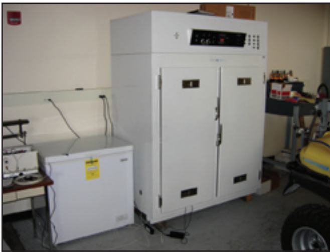
Figure A-1—A commercial freezer (left) was used for the extreme cold temperature tests. Cold startup and operation tests were conducted in the freezer at -15 °F.
