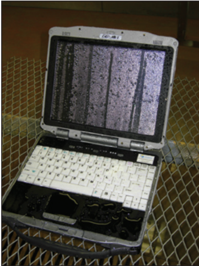
Figure 2—The laptops were tested for rain/moisture resistance. The laptops were sprayed for 10 minutes on each axis with a simulated rain of 4 in/h at 40 mi/h. Both laptops passed all rain/moisture tests.
