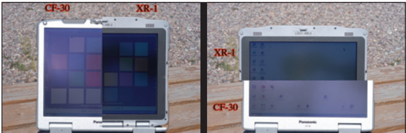
Figure 4—The laptops were compared side-by-side to determine how well the screen could be seen in direct sunlight. While the screen of the CF-30 laptop was brighter, the new DynaVue screen of the XR-1 laptop had better contrast and less glare, making it easier to view.
