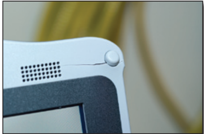
Figure D-1—A crack developed on the XR-1 laptop after one of the drops. The XR-1 laptop still functioned properly, but its integrity was compromised. The CF-30 laptop passed all drop tests.
