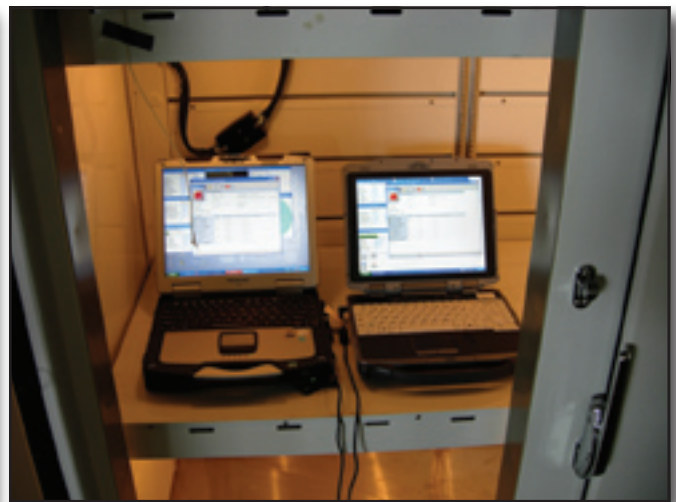
Figure B-2—Both laptops were placed in the environmental chamber for two h at 120 °F. Then they were started and tested.
