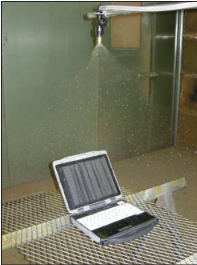
Figure C-1—The laptops were subjected to simulated rain to test their resistance to moisture. The laptops were sprayed for 10 minutes on each axis with a simulated rain of 4 in/h at 40 mi/h. During one test the laptop was open while the screen and keyboard were sprayed.
