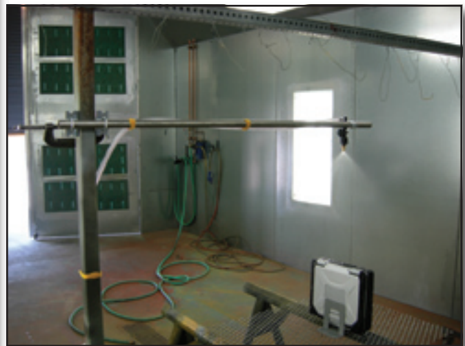
Figure C-2—The nozzle was suspended on a pole mounted to a metal frame. The pole could be adjusted so that the nozzle was 48 cm above the laptop.
