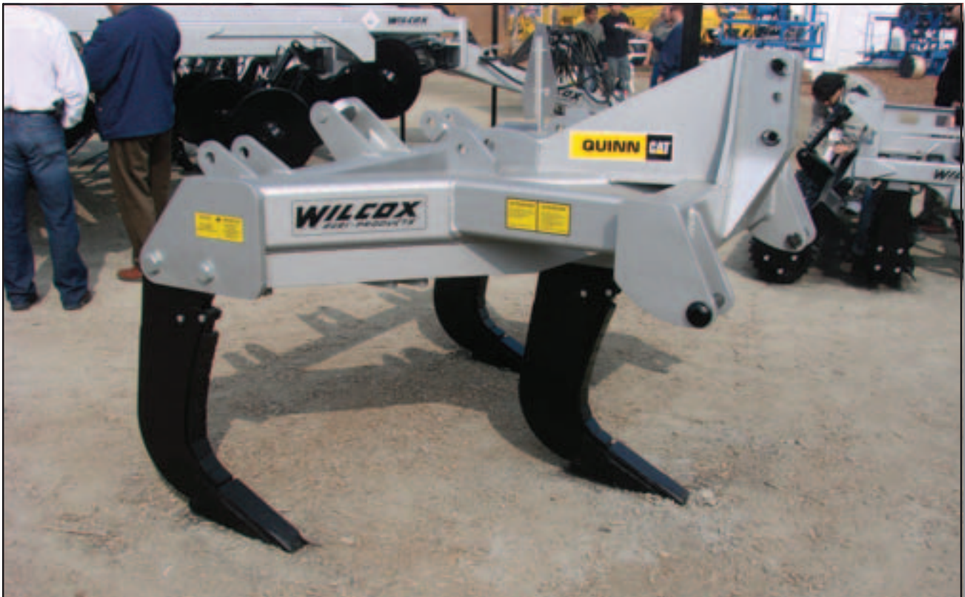
Figure 1—This three-shank subsoiler attaches to a tractor's three-point hitch. It can fracture compacted layers 12 to 22 inches below the soil surface.
