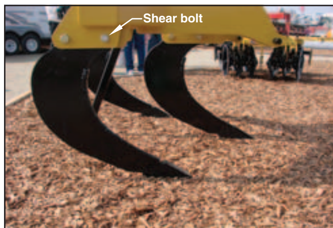
Figure 5a—Shanks need to be mounted to subsoilers so that the shank can survive if it runs into rocks or stumps. The shank above is protected by a shear bolt designed to break if too much force is put on the shank.
