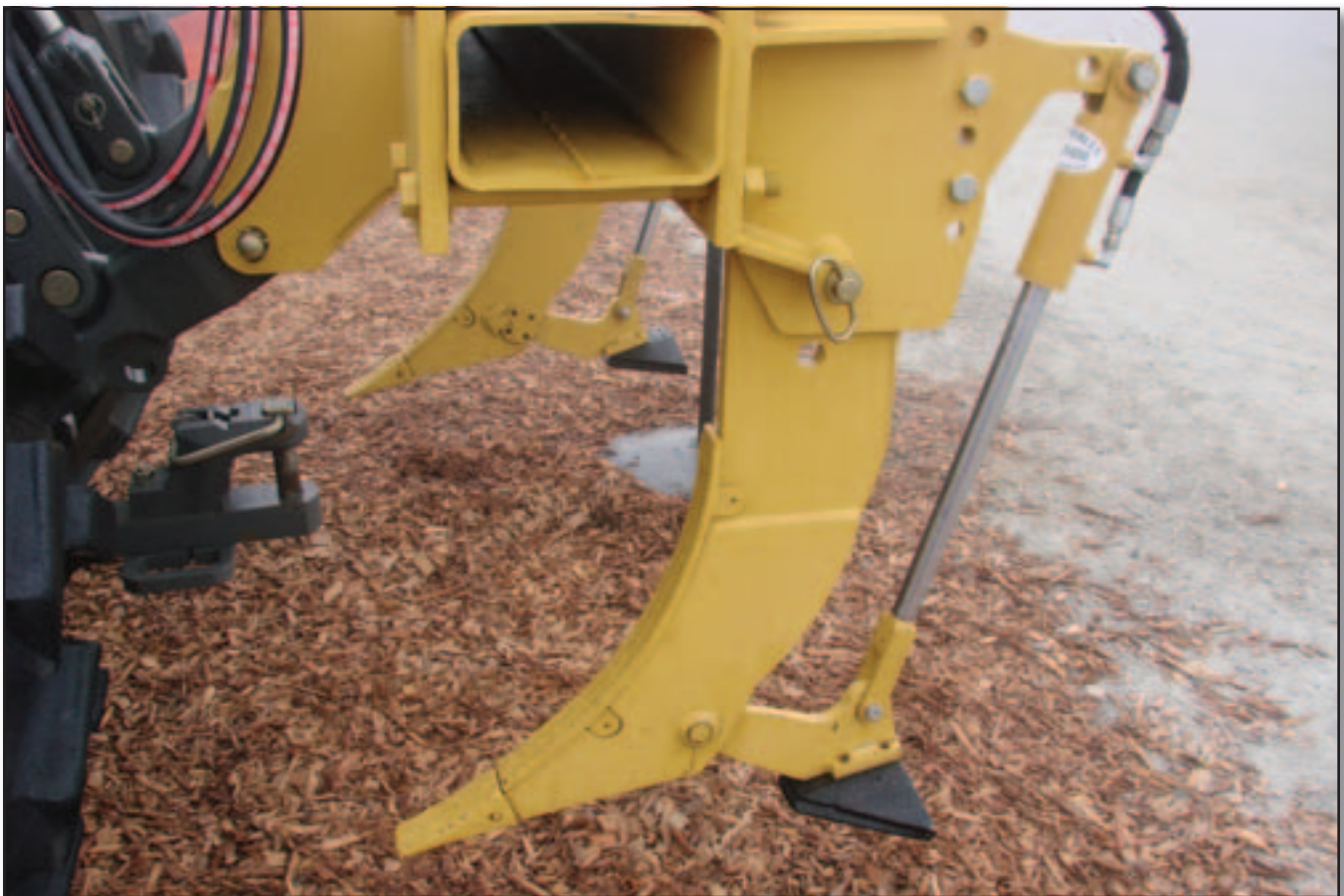
Figure 11—The wing on this subsoiler moves up and down with a hydraulic ram mounted behind the shank.
