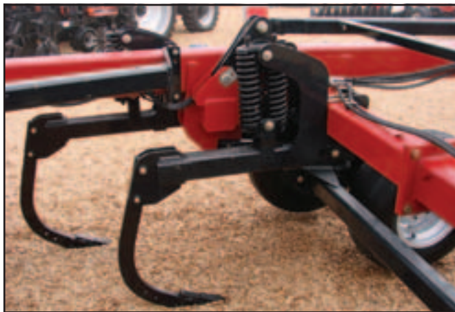
Figure 5b— This photo shows shanks with springs that allow them to pull back when they strike an object, resetting themselves once they have cleared the object.
