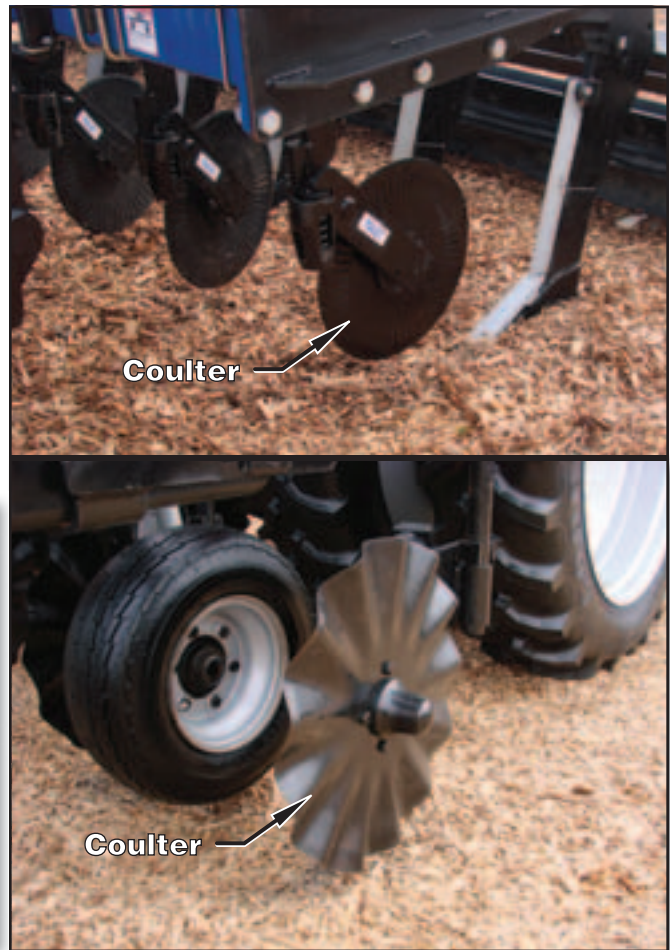
Figure 6—Coulters help cut slash and other surface residues so they don't hang up in front of the shanks. The coulters can be straight (top) or fluted (bottom).
