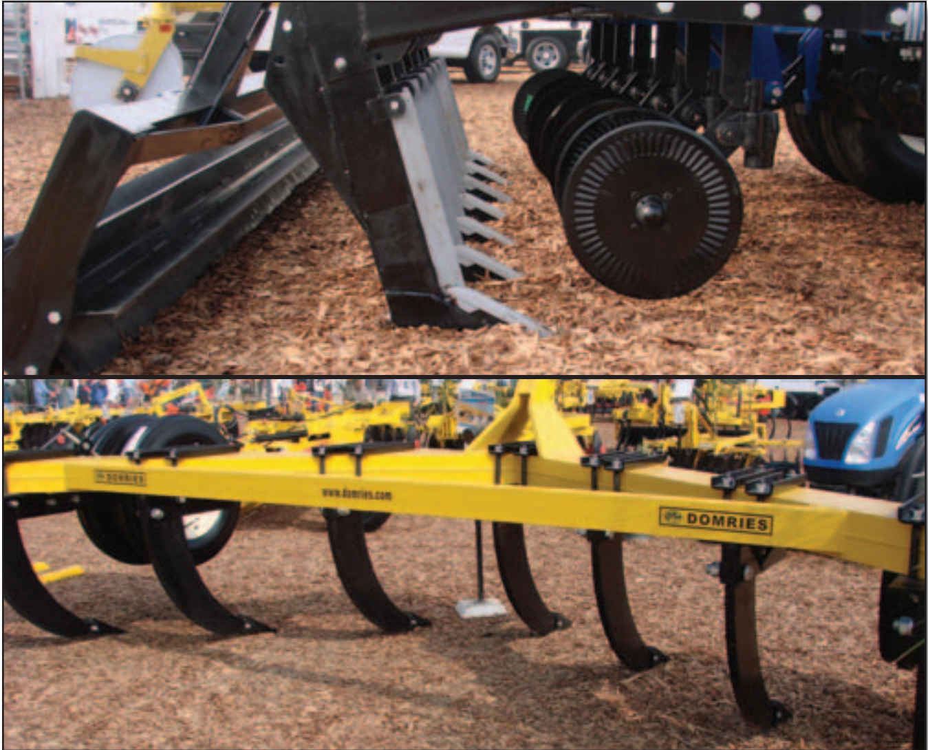
Figure 7—Shanks can be attached to the subsoiler frame or toolbars in a straight line (top) or in a V-shape (bottom).
