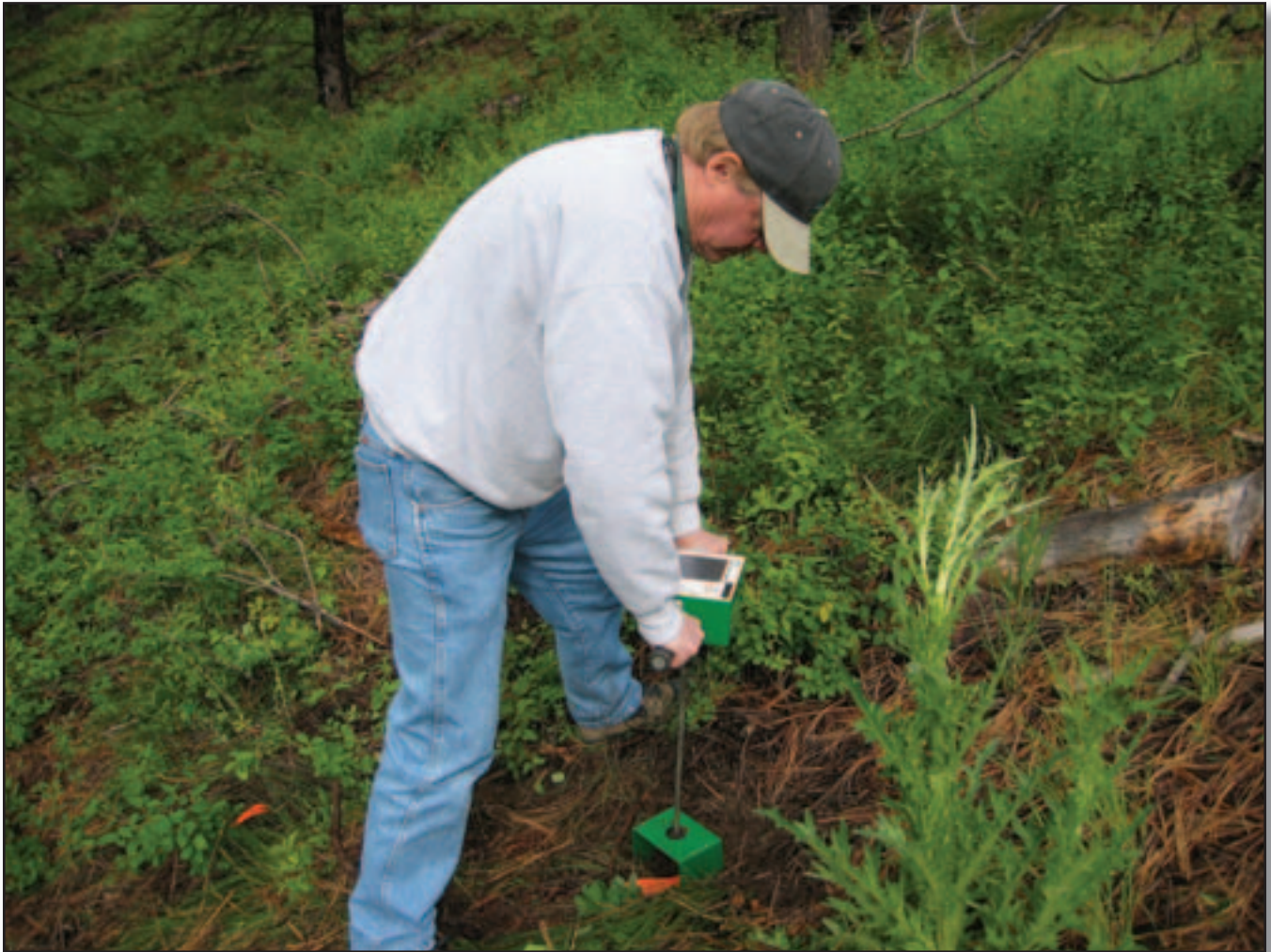
Figure 10—Soil penetrometers can be useful when determining whether soil layers have been compacted or when checking to see how well areas have been fractured by subsoiling. Penetrometers don't work well in areas with lots of rocks or roots.
