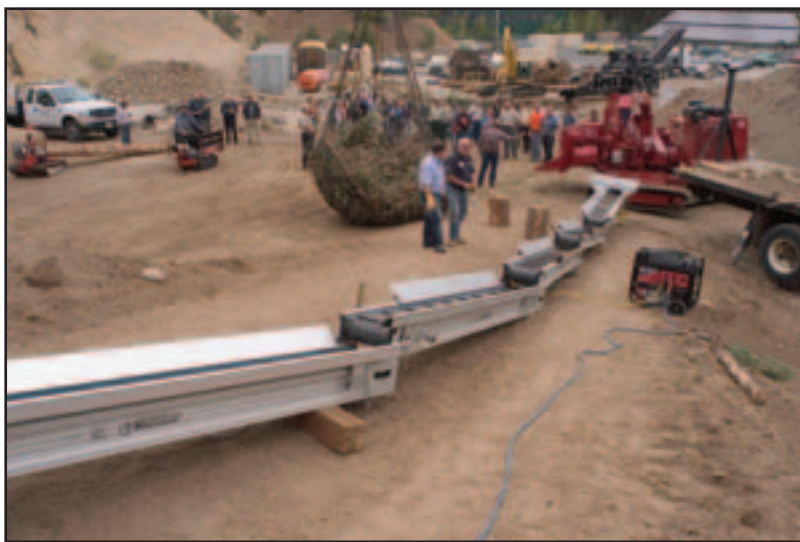
Figure 1—Early tests using a portable conveyor to remove slash were conducted in a gravel pit in Incline Village, NV.
