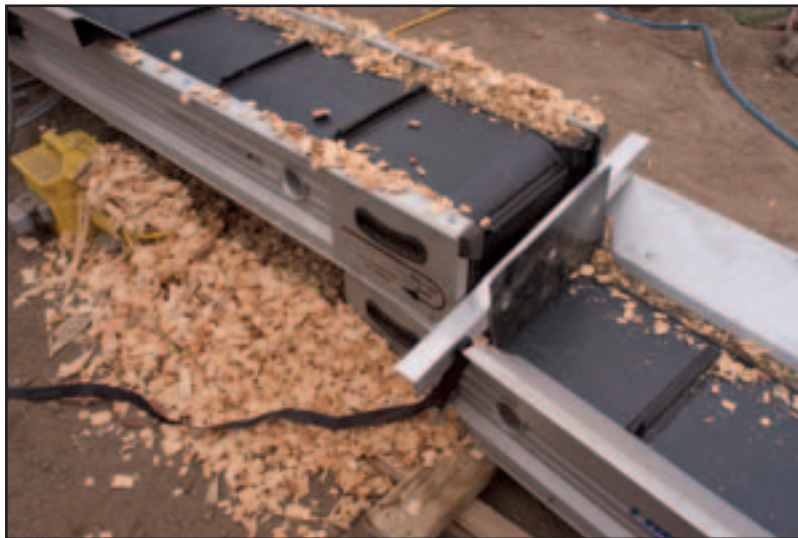
Figure 3—Chips fell from gaps in the conveyor's side extensions.
