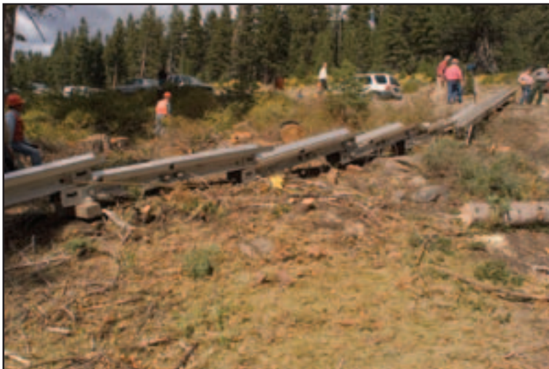
Figure 2—When the conveyor was set up in the woods for a more realistic test of slash removal, the conveyor sections were overlapped.
