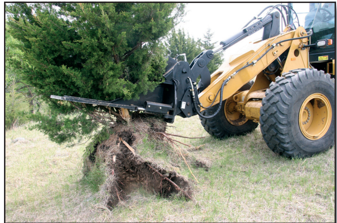
Figure 17b—Star Hill Super JAWZ with adapter for Caterpillar 924 (Photo courtesy of Starhill Solutions, Inc.).
