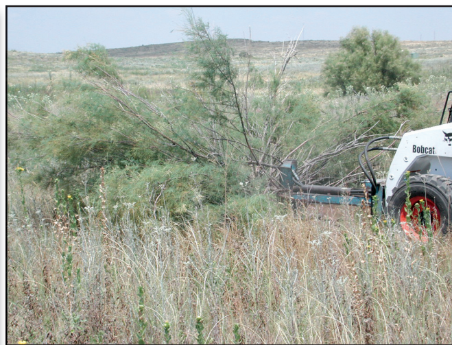
Figure 9c—The Bobcat brush saw being used to cut tamarisk.
