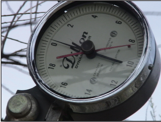
Figure 2—A Dillon 20,000-pound dynamometer used to determine how much force was needed to pull tamarisk.
