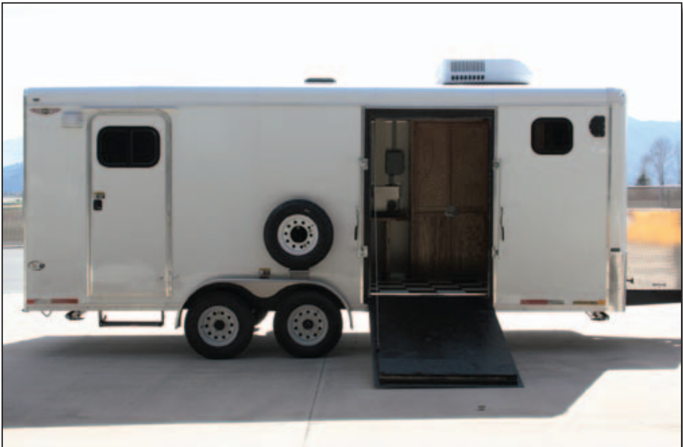
Figure 1—The MIMIT trailer provides a secure and environmentally protected space for the server and other equipment. The trailer and IT equipment are configured before incidents so they can be deployed and set up rapidly. The trailer also provides a working space for the incident's computer technical specialist and other incident personnel.
