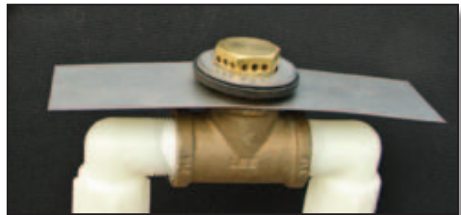
Figure 6—A thin stainless steel plate under the water feed nozzle helps distribute the weight of the heavy brass fittings.
