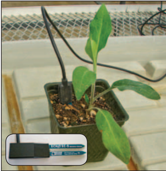
Figure 4—An ECH2O EC-5 soil moisture sensor, manufactured by Decagon Devices, Inc. (inset), is inserted into the potting soil in one of the container plants.
