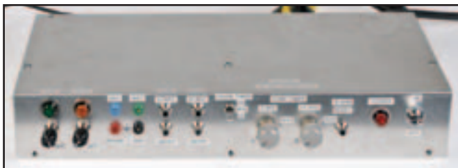
Figure 7—The automated subirrigation controller.
