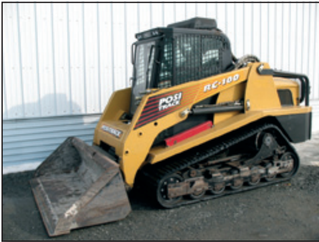
Figure 1—The ASV Posi-Track Compact Track Loader (a skid steer) is used by the Klamath National Forest's Goosenest Ranger District for many timber stand improvement projects. Because skid steers are supported by tracks, they cause very little soil compaction.
