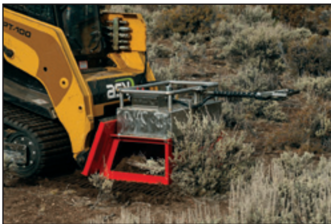
Figure 2—MTDC developed a torch that attaches to an ASV skid steer. The torch, which mounts on a standard skid steer universal attachment plate, burns a mixture of diesel and gasoline. Many safety features have been incorporated into the torch.
