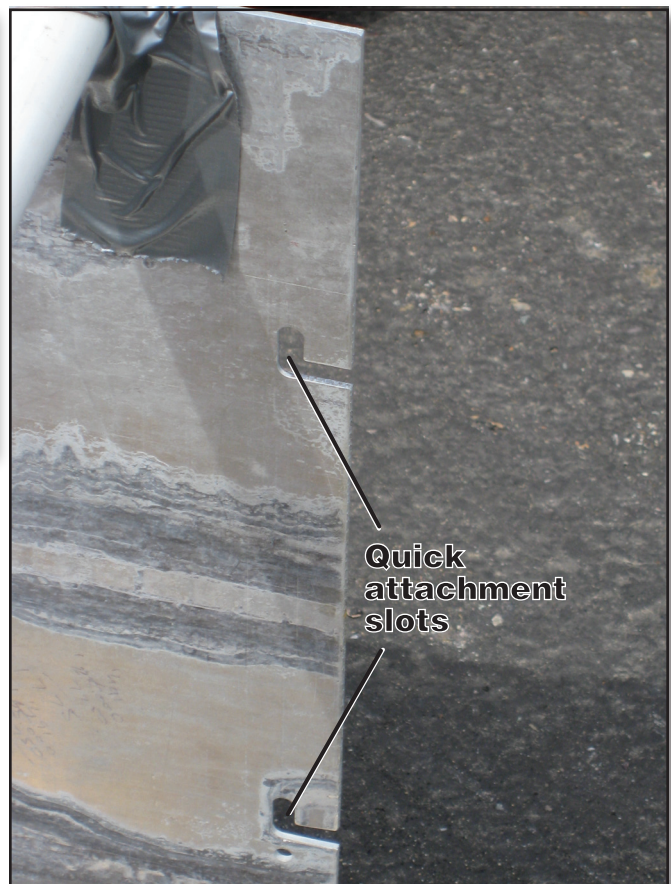
Figure 12b—The debris collection bin's quick attachment slots.
