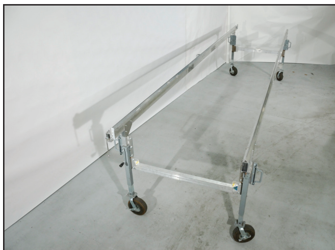
Figure 4b—Both jack stand assemblies are attached to the rails.
