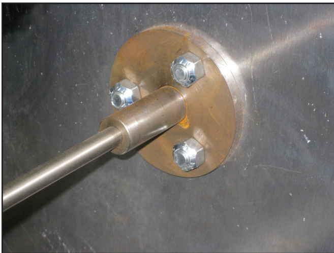
Figure 19—Three bolts must be removed to change the reel paddles.
