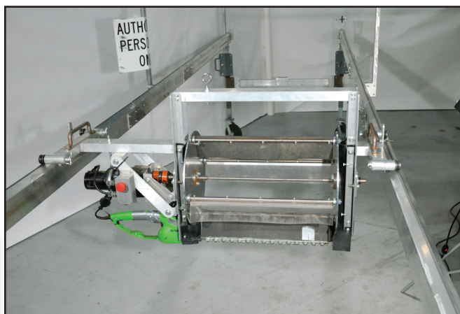
Figure 8—Two people are needed to place the cutter/reel assembly safely on the top pruner's rails.
