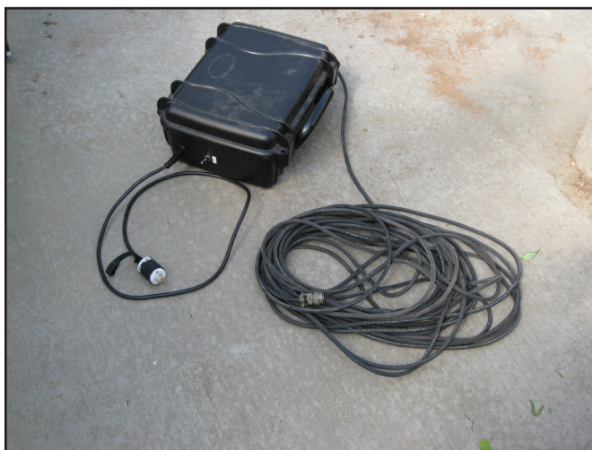
Figure 13b—The waterproof plastic voltage transformer box.
