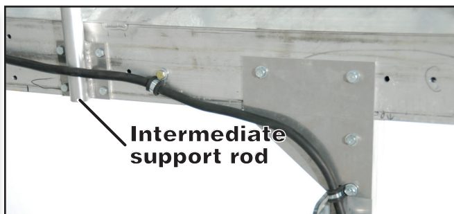
Figure 10g—The electrical wire is routed around the intermediate support rod.
