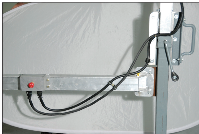
Figure 10d—Routing the electrical wires into the kill switch.
