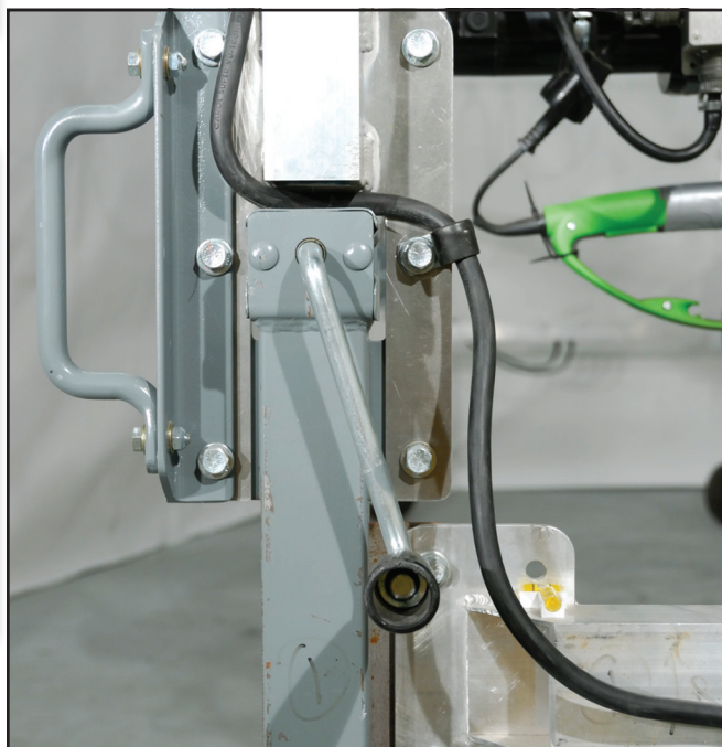
Figure 10h—The electric wire is routed above the crank handle on the master control box end of the top pruner.
