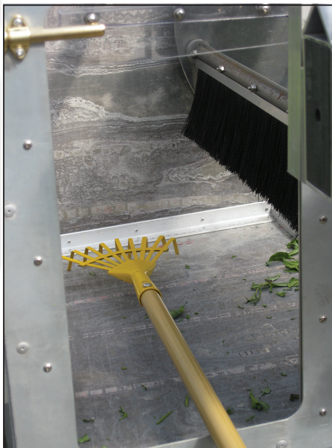
Figure 18b—Use a short rake to pull the cut tops from the collection bin into a cardboard box or trash can lined with a garbage bag.
