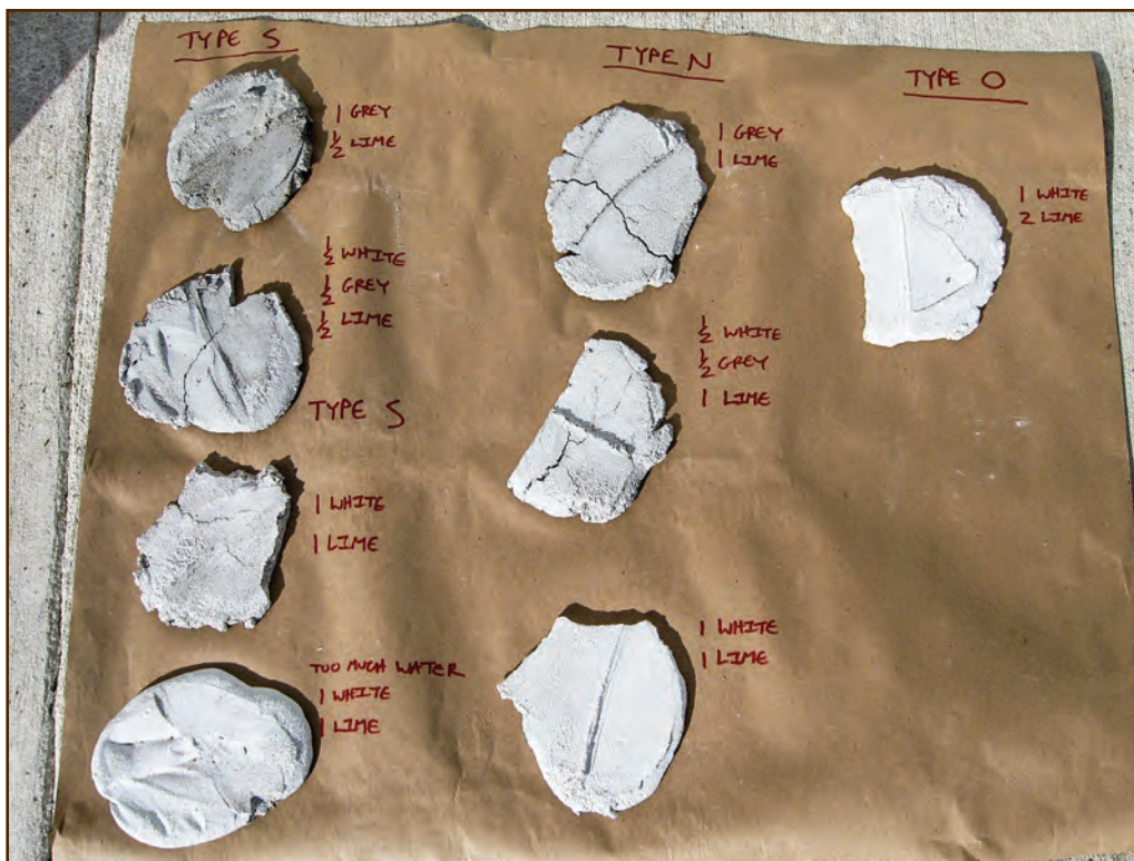
Figure 196—These mortar samples show the difference in appearance when you make mortar using various combinations of lime and white or gray cement. The preservation specialist used the same sand and water for all the samples.
