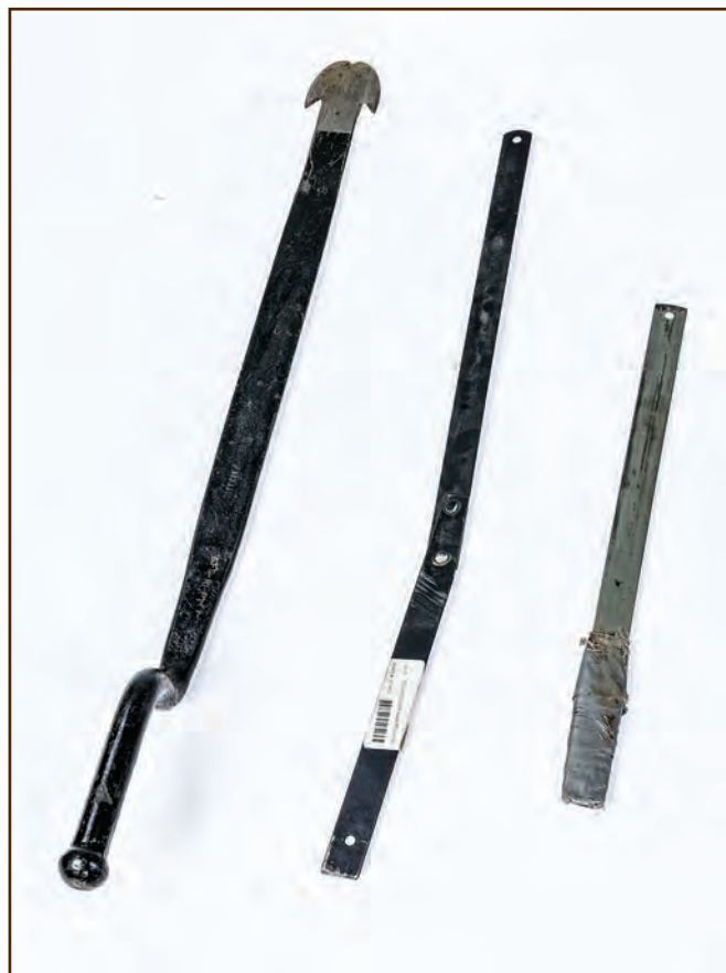
Figure 232—You can slip a shingle ripper (left) up under a shingle and around a nail, then hammer down sharply to cut the nail. You also can slip a roofer's saw (right two) under a shingle and use the tiny teeth to saw the nails. Either tool will sever roofing nails so that you can remove individual shingles without damaging the surrounding shingles.
