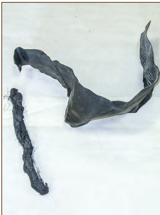
Figure 240—The lead on the left is lead wool. You can use it to pack the joints behind the mortar in a chimney and hold the flashing in place. The lead on the right is used lead sheet flashing.
