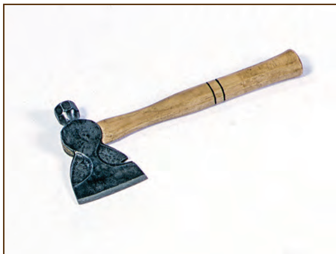
Figure 257—This older shingling hatchet serves the same function as newer models—use the hammer end to drive nails, the hatchet end to trim shingles, and the notch in the hatchet to pry out nails.
