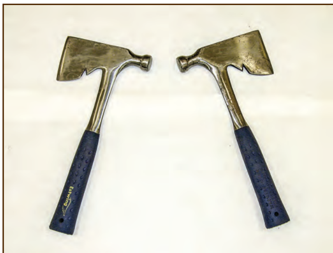
Figure 258—These newer shingling hatchets work exactly the same way as the older hatchet shown in figure 257. Their steel handles are less likely to break, but the basic design hasn't changed much in more than 100 years.
