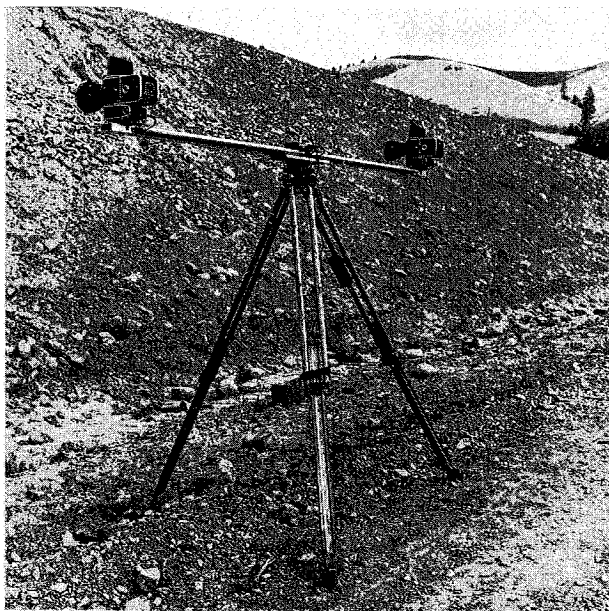
Figure 1.--Electrically driven cameras on 2-m mounting bar.
