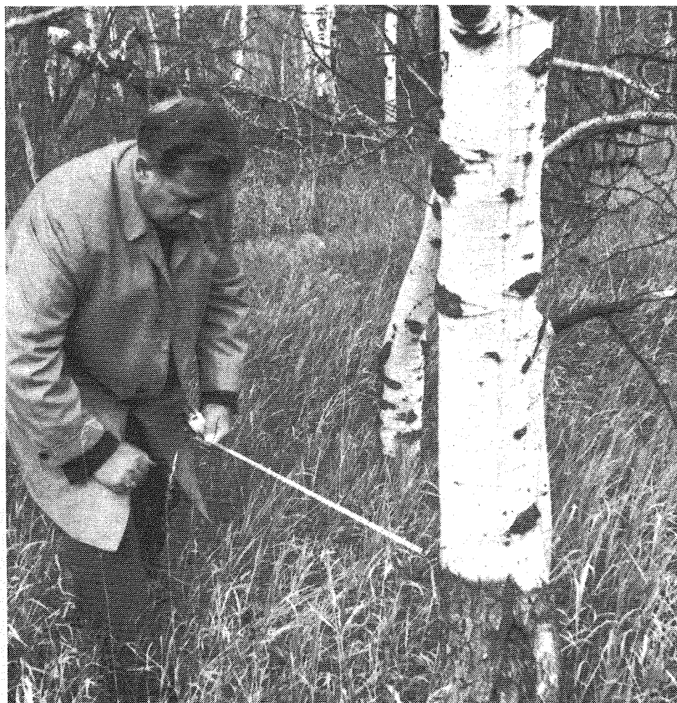
Figure 3.--Olson hooks tape measure to nail in tree to measure changes in distance.
