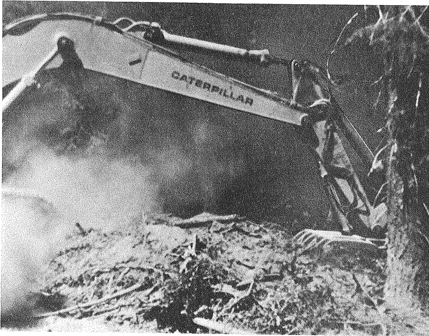
Figure 5.--Clam shell grubbing brush.
