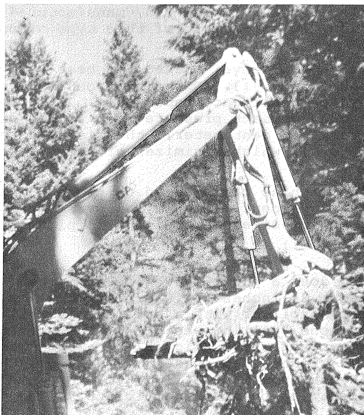
Figure 2.--Hydraulically activated clam shell.
