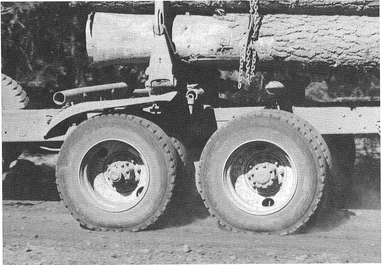
Figure 2.--Radial tires with lowered air pressure produce less stress on the road surface.
